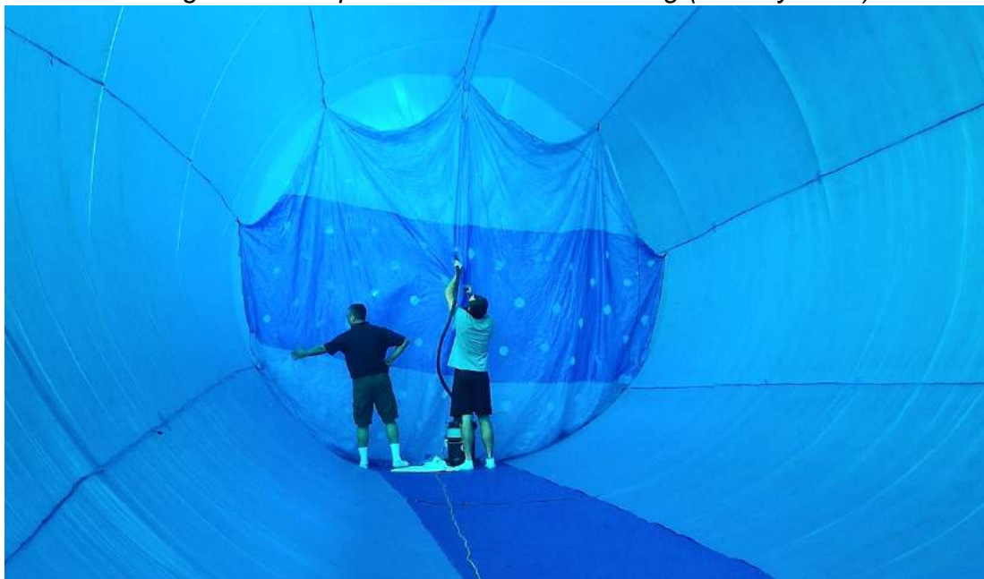
17.1 ft (5.2 m) diameter outer envelope with divider wall being installed. Source: JPA blog (posted 14 Feb 2017)
