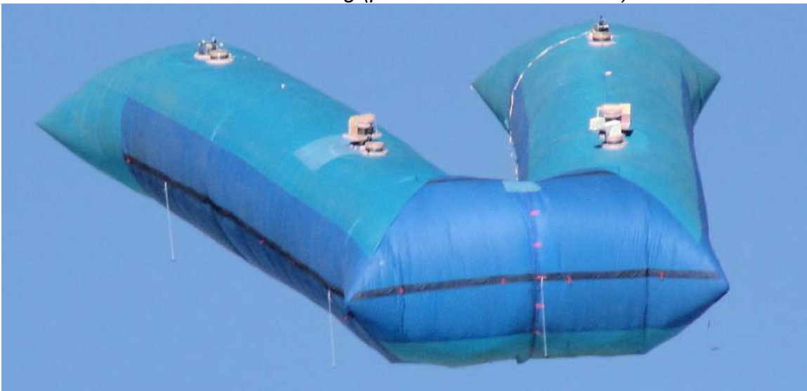
Ascender 26 in flight, showing the top deck and valve / fan locations. Source: JPA blog (posted 20 July 2015)
