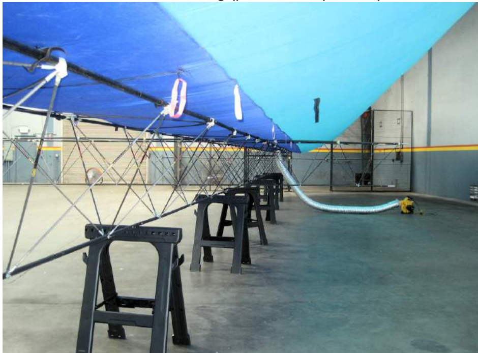
Closeup view of an 80 ft (24.4 m) long external carbon fiber keel truss on Ascender 9. Source: JPA blog (posted 29 July 2017)
