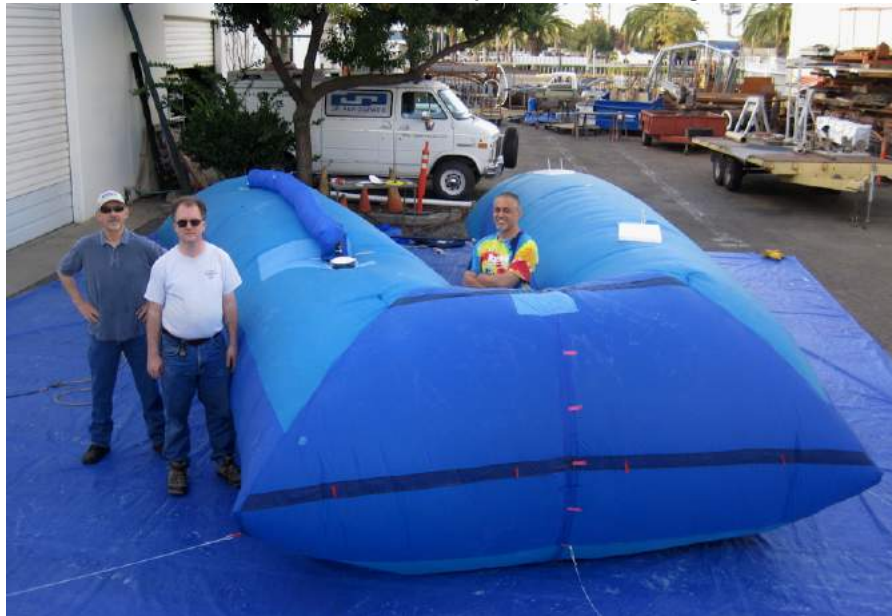
Ascender 26 with the starboard helium transfer tube (dark blue) installed on the top of the outer envelope (two-tone blue).
