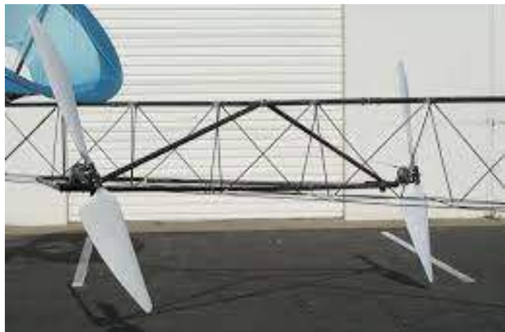
Left & below: The battery-powered, electric motor-driven, twin propellers are optimized for operation at very high altitudes. Source, two photos: JPA
