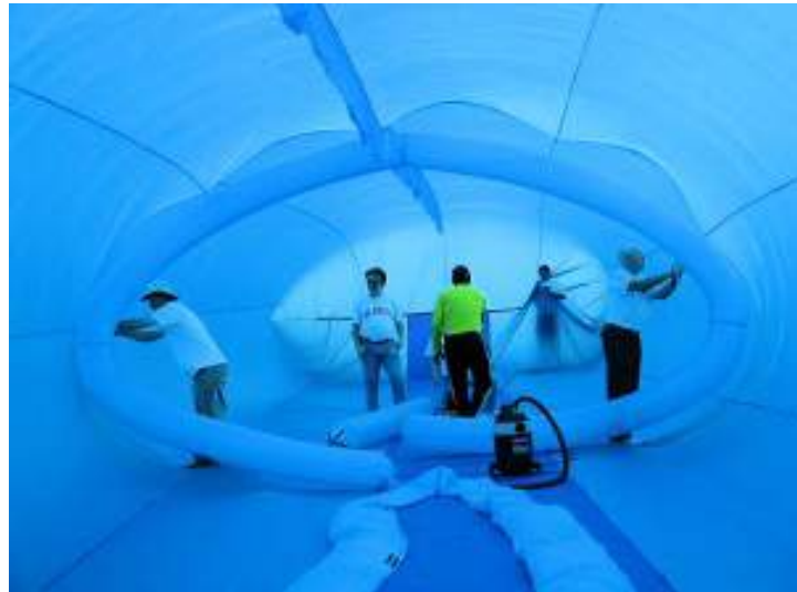
Air beam used as Ascender wing rib structure. Source, both photos: JP Aerospace Blog (5 March 2018)
