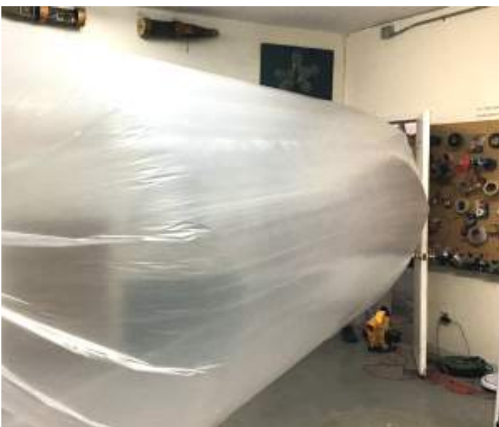
The first manufactured helium lifting gas cell for the Ellipse. The airship will have a total of four helium lifting gas cells. Source: JP Aerospace Blog (23 August 2023)
