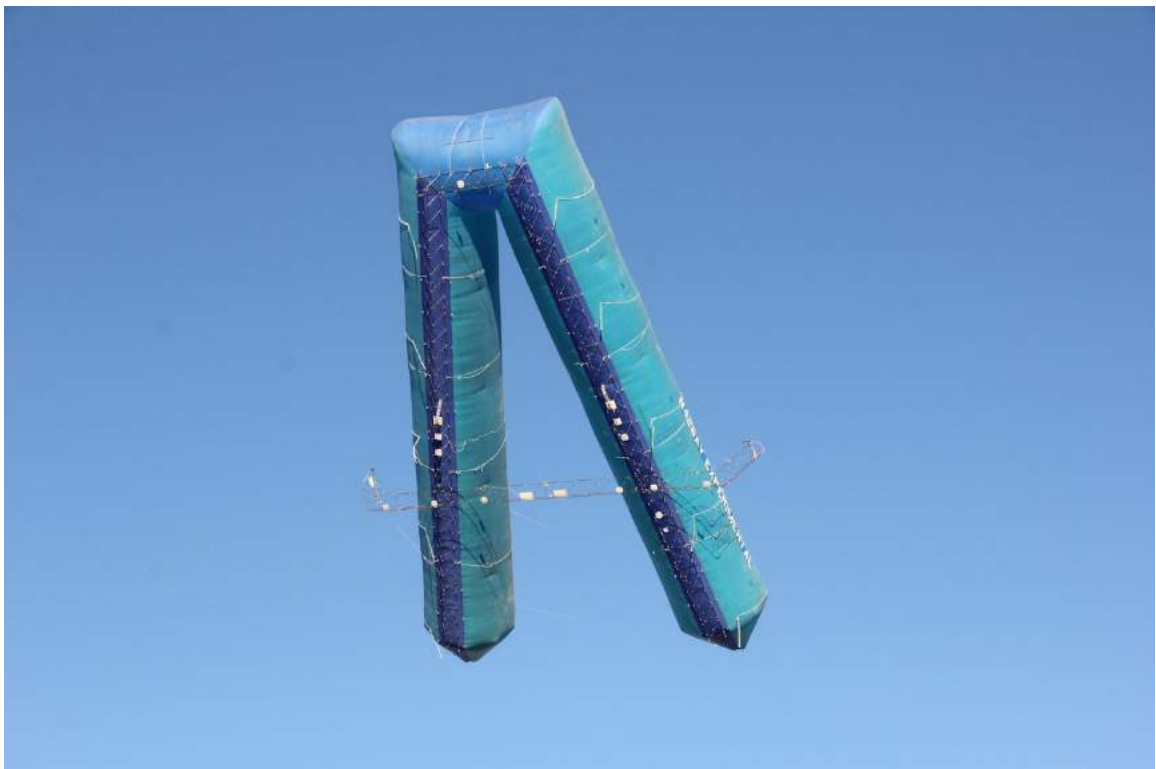
Ascender 9, viewed from below after launch, showing the external truss structure. Note that the propellers are at the ends of the diagonal arms extending from the cross-beam, outboard of the arms of the V-shaped envelope. Source: JPA.
