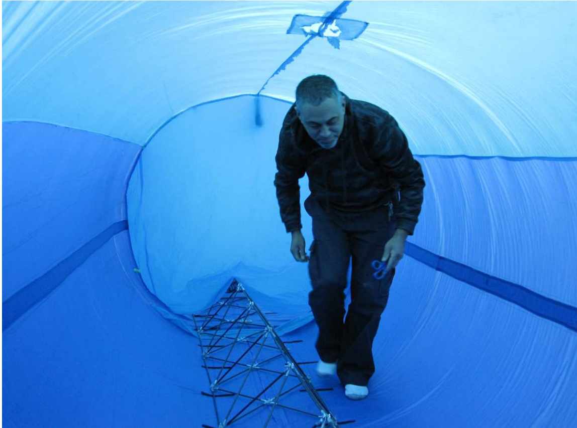
Inside the inflated outer envelope, showing an internal cell divider wall and the internal keel structure. Source: JPA blog (posted 2 December 2013)
