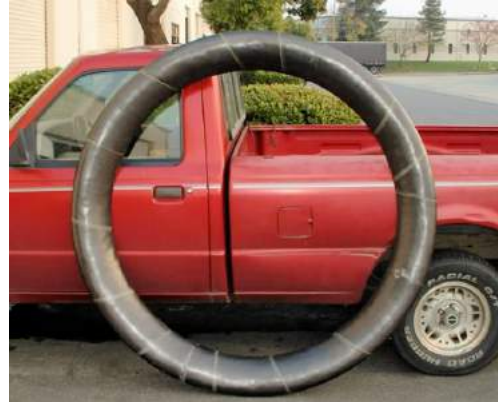
(Left) General arrangement of the carbon fiber structural ring. (Right) Ring shown to scale with a pickup truck.
