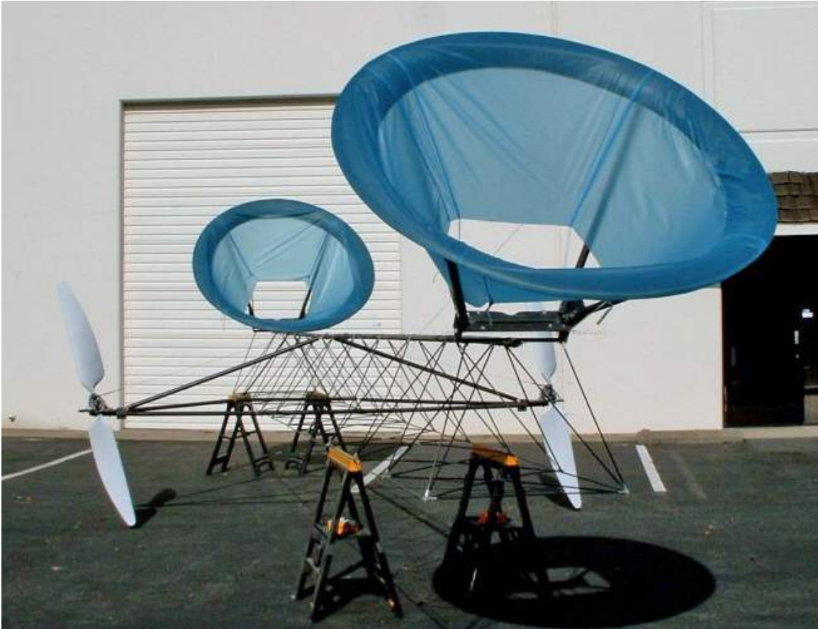
Above: Tandem Airship has a triangular section carbon fiber cross-beam with two mating cones (blue) for connecting the twin superpressure balloons to the airship structure. Source: JPA
