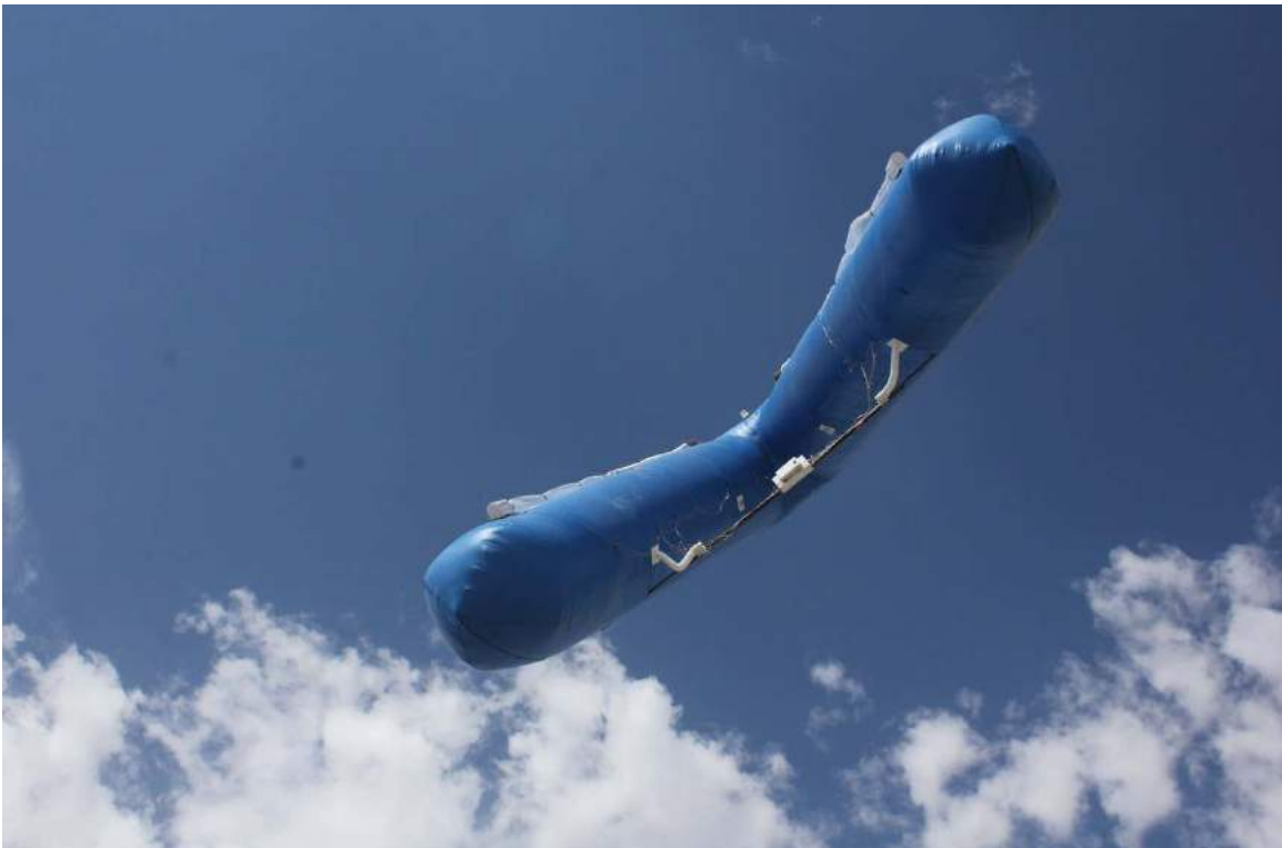
Ascender 36 in flight, view from behind showing the cross-beam, propellers & payload pod. Source: JPA
