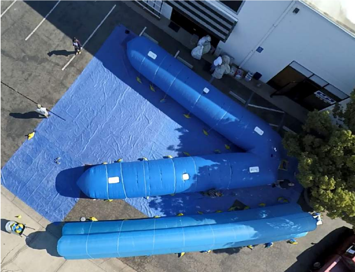
Ascender 36 final ground inflation and system testing with all airship systems installed except the rigid cross-beam and propulsion system, prior to first flight. Source: JPA (August 2016)
