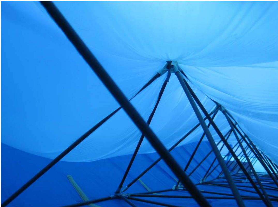
Ascender 26 internal carbon fiber keel structure is held in place with Velcro straps. Source: JPA blog (posted 10 November 2014)
