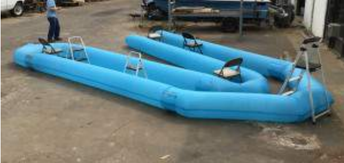
Airbeams inflated prior to installation on the Ellipse. Source: Source: JP Aerospace Blog (2 October 2022)
