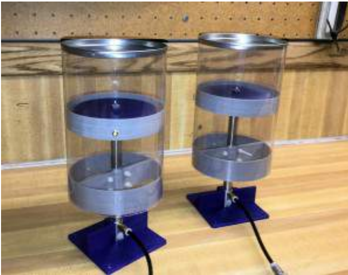
Ascender actuated helium valves (left) and being tested at high altitude on the Away 129 mission (below). After further testing, the valves are intended for the Ellipse II airship (formerly Ascender 48). Source, both photos: JP Aerospace Blog (27 February 2020)
