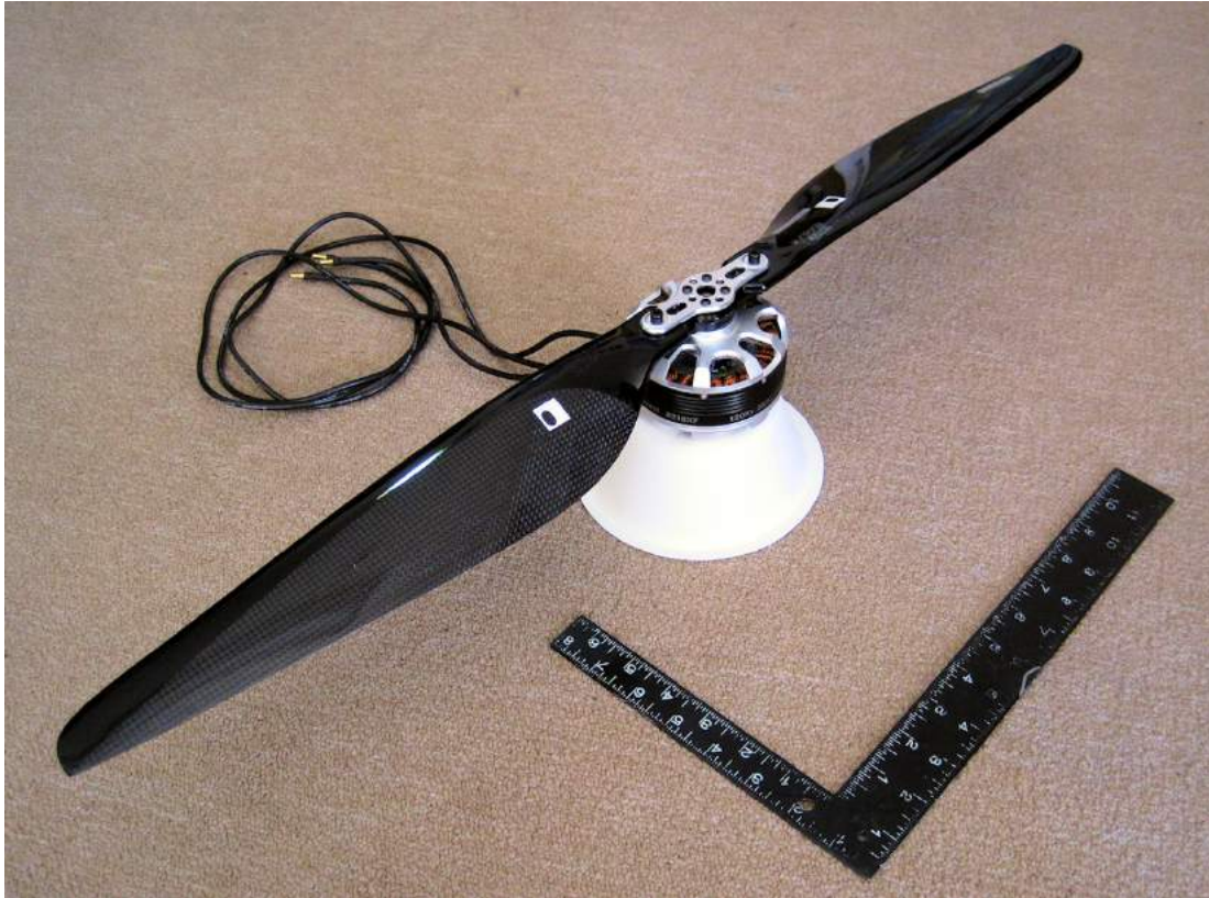
Ascender 9's KDE8218XF very high-efficiency, 28-pole, brushless electric motor manufactured by KDE Direct, and a two-bladed carbon fiber propeller optimized for high altitude operation. Source: JPA blog (22 May 2017)
