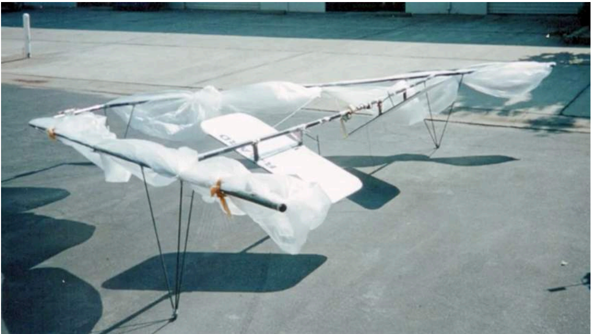
Mylar lifting gas cells attached to an aluminum framework. There was no outer envelope. Source, both photos: Screenshot from JPA video (1 Nov 2022)
