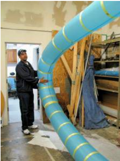
Air beam used as Ascender wing rib structure. Source, both photos: JP Aerospace Blog (5 March 2018)
