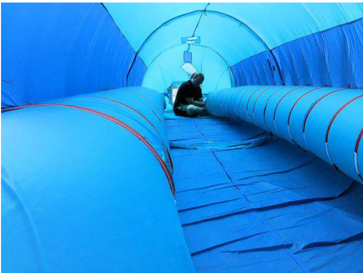
Airbeams secured with straps to the shell of the Ellipse. Next step in vehicle assembly is to test fit the helium lifting gas cells. Source, both photos: JPA Facebook (5 August 2023)
