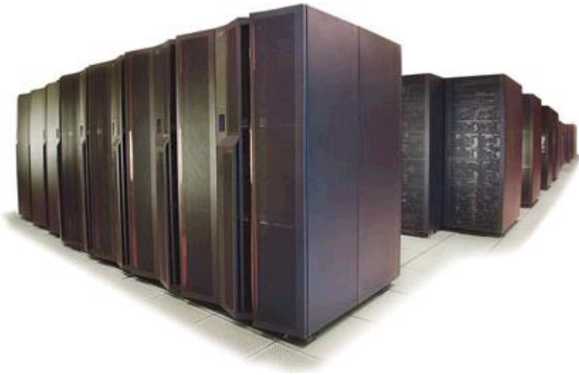
IBM Power4 Data Star 2000 cpu, 17 Tflops GPFS filesystem
