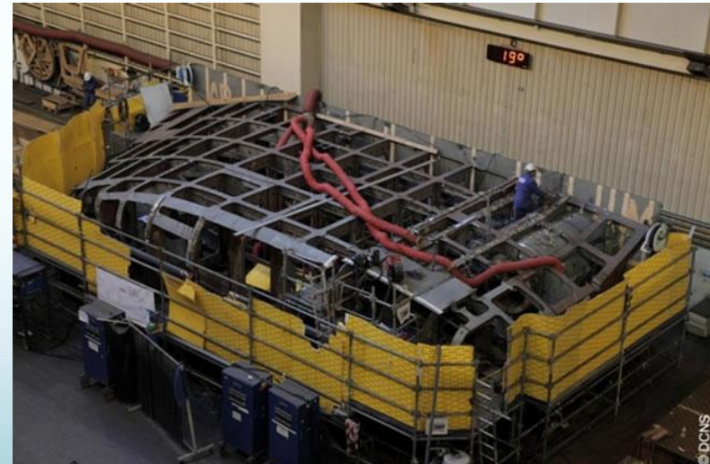
Barracuda sail under construction. Source: DCNS
