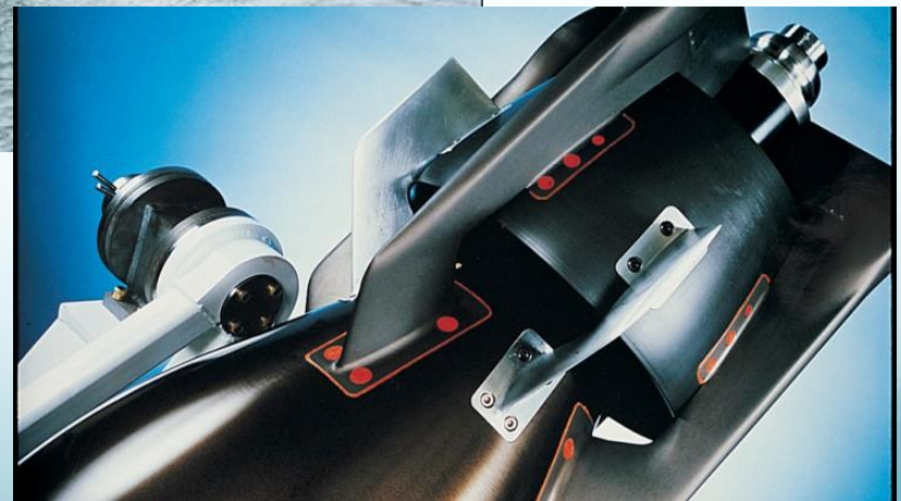
The Spearfish pumpjet propulsor. Source: https://www.thinkdefence.co.uk/2014/11/spearfish-torpedo-upgrade/
