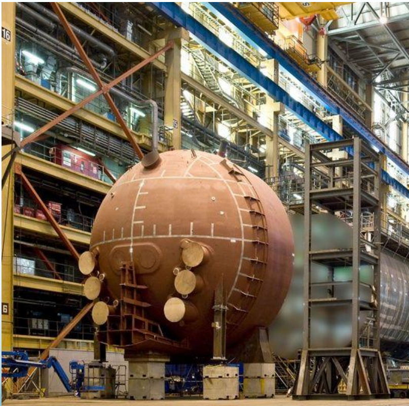
Sub on left: Bow pressure hull closure dome with penetrations for six torpedo tubes. Source: http://www.naval-technology.com/
