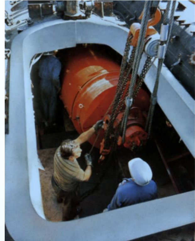
Large equipment being handled through a brèche on SSN Améthyste , with a protective combing over the seating surface. *
