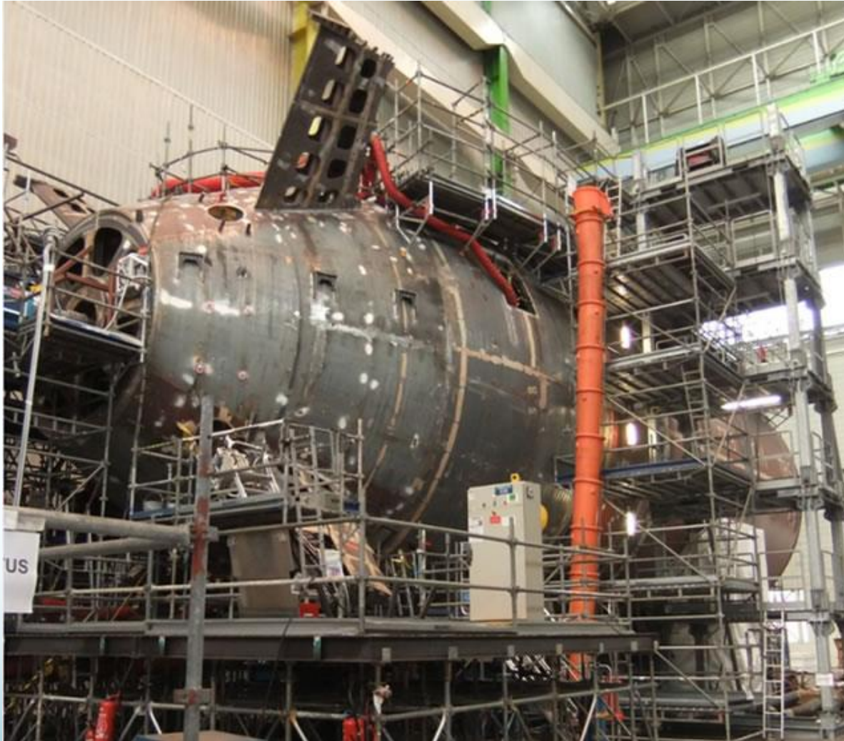
Barracuda stern section showing X-control surfaces. Source: DCNS
