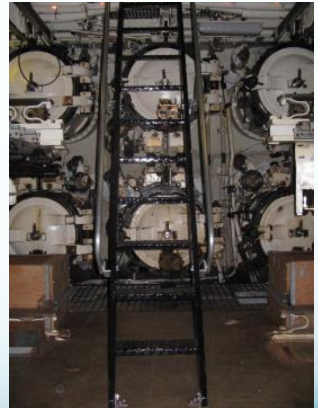
Torpedo room, 6 bow torpedo tubes
