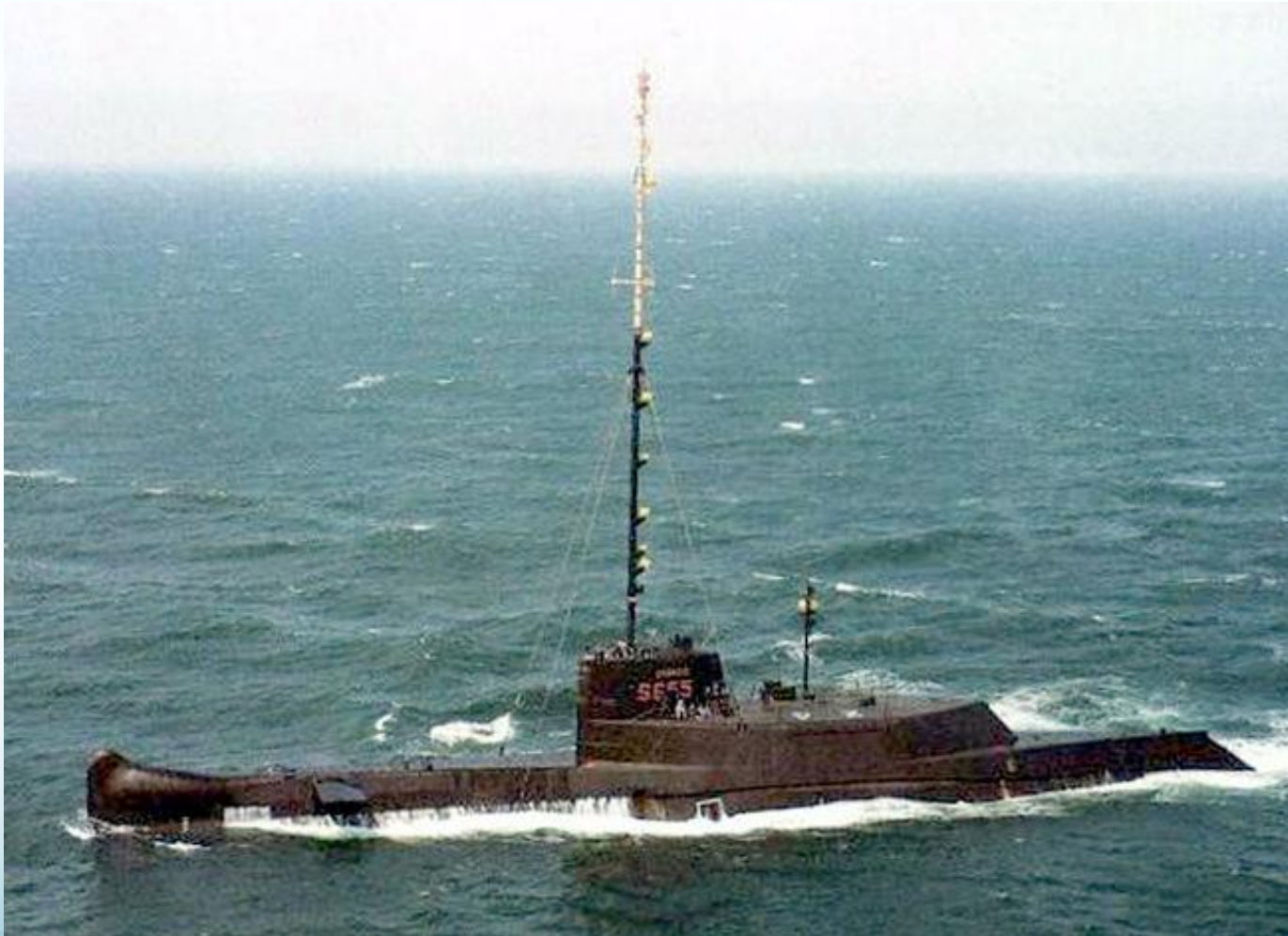
Gymnôte 2 with telemetry mast for underwater launch test.
