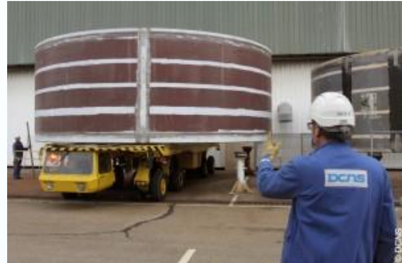
Barracuda hull segment being moved. Source: DCNS
