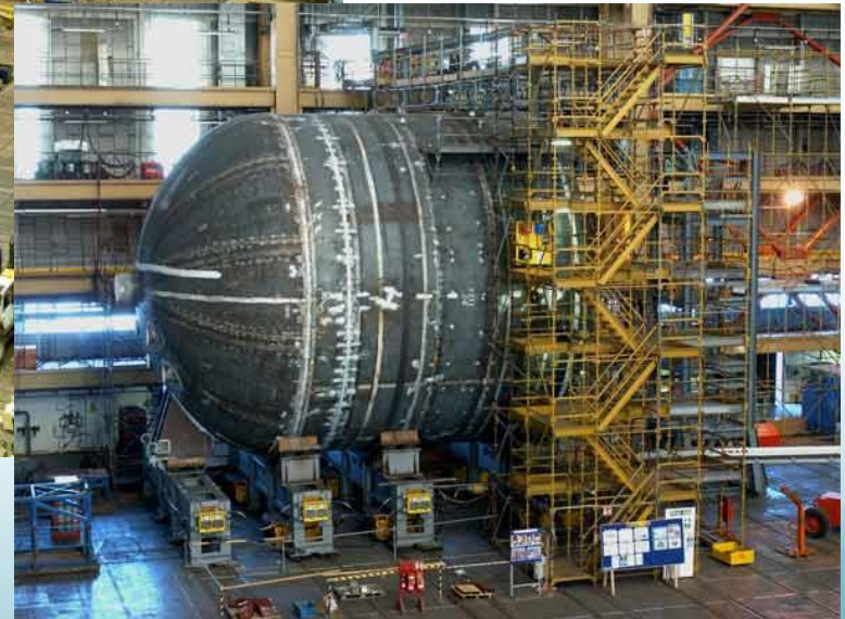
Below: Stern pressure hull segment. Note the propulsion shaft penetration in the center of the closure dome. Source: http://www.naval-technology.com/
