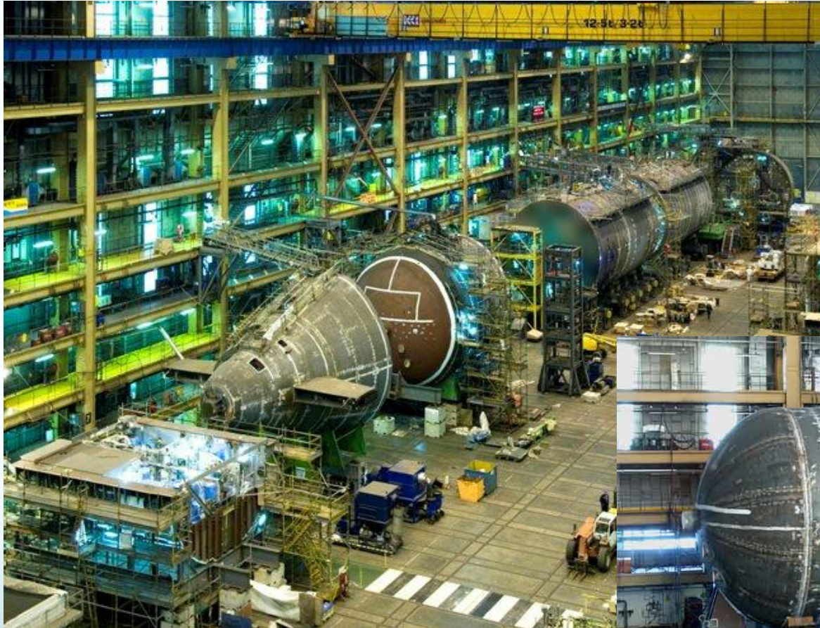
Above: Stern cone aligned with stern pressure hull closure dome.
