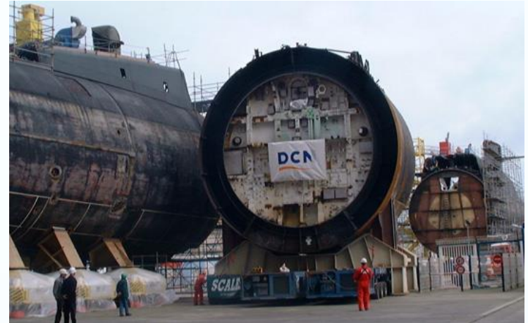
Reactor compartment removed. Source: DCNS
