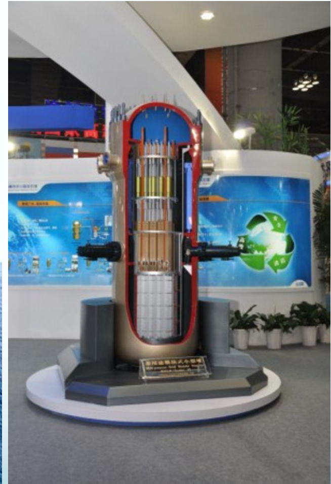
CNNC ACP100+ integral PWR reactor. Source: China National Nuclear Corporation
