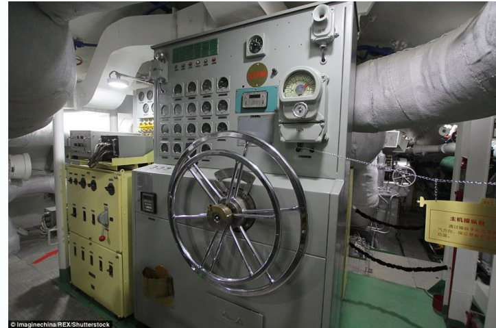
Above: Throttle control panel (ahead & astern throttle wheels) Below: Passageway beside the reactor compartment
