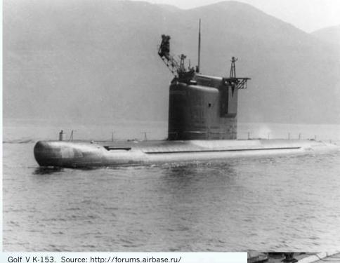
Equipped with a single launcher in the sail to carry out tests of the R-39 SLBM for the Typhoonclass SSBN.
