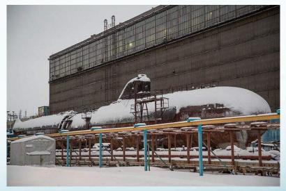
K-3 after cuts in the hull were made to remove the reactor compartment. Source: http://www.subsim.com/ radioroom/
