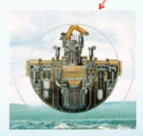
The above diagrams from the Gidropress website likely shows a cross-section of the BM-40A reactor within the outline of an Alfa submarine hull.
