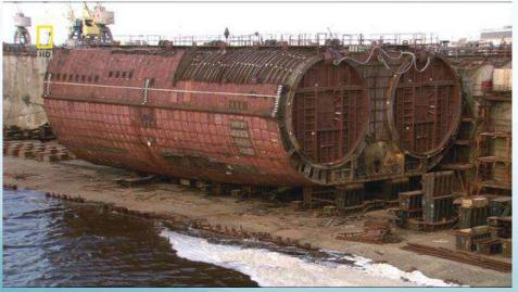
Typhoon reactor compartment removed and sealed. Source: Pinterest
