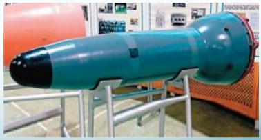
One reentry vehicle of a three-RV cluster warhead.
