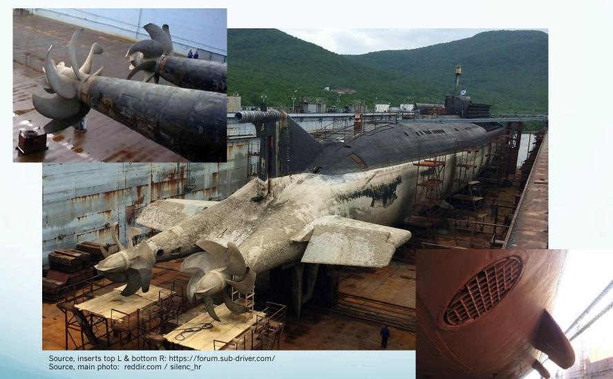
Seawater coolant inlet scoops and discharge.
