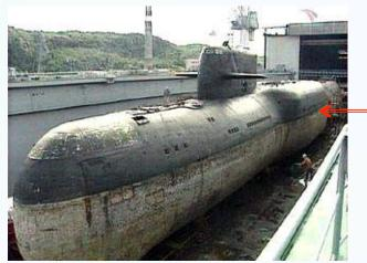
"Sidecar" for mid-ships SS-N-24 cruise missile launchers outside the pressure hull
