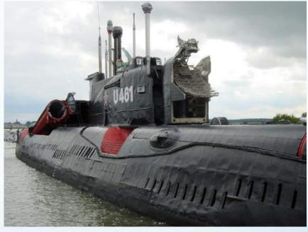
Above: Large guidance antenna for anti-ship cruise missile midcourse guidance was built into the forward edge of the sail structure, which opened by rotating.
