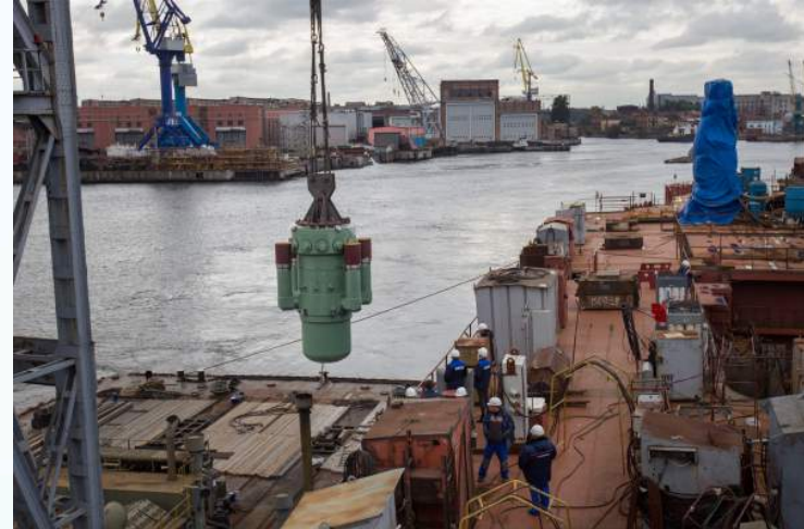
RITM-200 being loaded on Arktika in Sep 2016. Source: http://www.navyrecognition.com/
