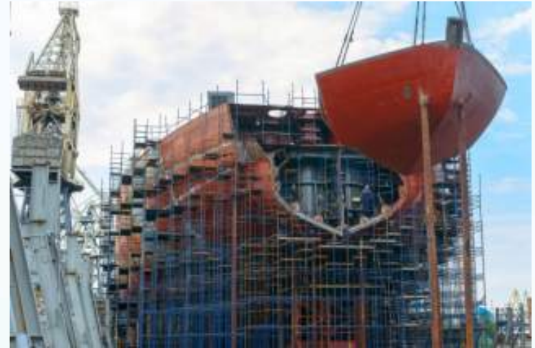
Arktika 's bow installed Aug 2015. Source: http://bellona.org
