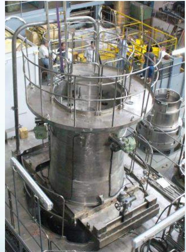
Refueling complex for a KLT-40 reactor on the floating power unit Akademik Lomonosov .
