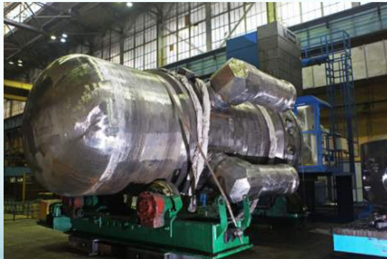
Right: Integral reactor vessel for 2 nd reactor on Arktika , with primary pump housings installed. Source: Rosatom
