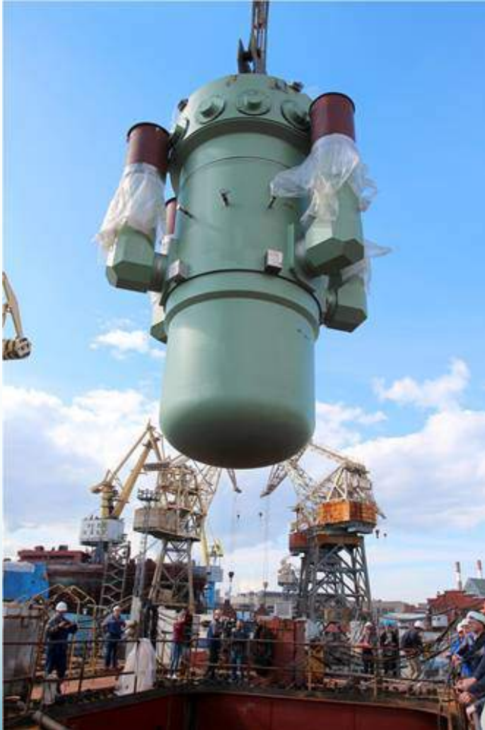
RITM-200 being loaded onto Arktika in Sep 2016. Source: https://www.marinelink.com/news/
