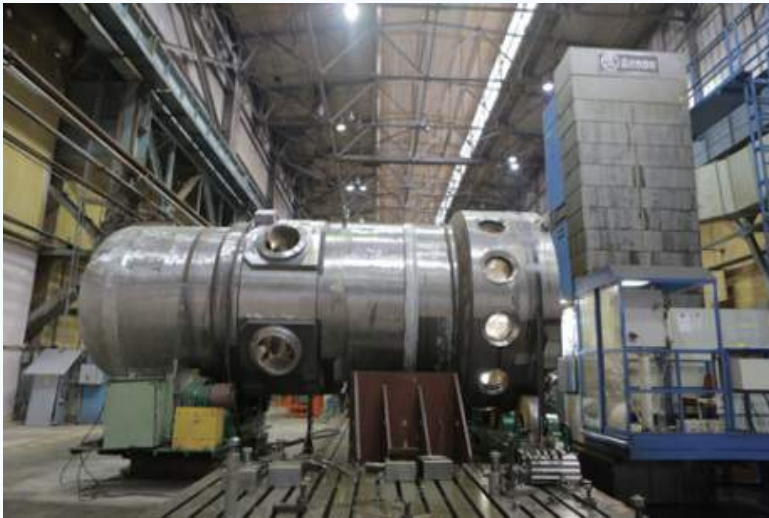
Above: Integral reactor vessel for Sibir before adding primary pump housings Source: Atomenergomash
