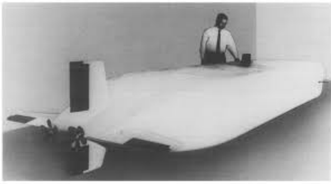
Submarine supertanker model: Source: L. R. Jacobsen & J. J. Murphy, "Submarine transportation of hydrocarbons from the Arctic", 1983
