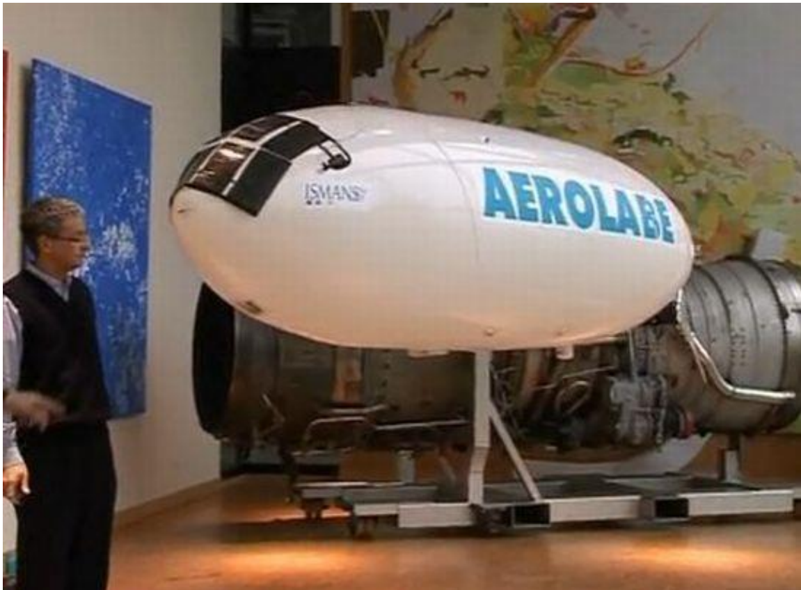
1/12 th scale model of the Aerolabe gas envelope before attaching the wing and tail. Source: screenshots from video.
