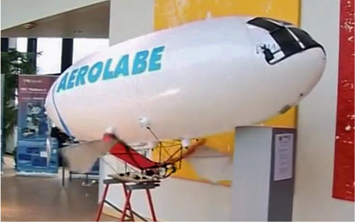
1/12 th scale model of the Aerolabe with the ornithopter mounted beneath the gas envelope. Source: screenshots from video.
