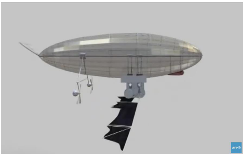
Propulsion via ornithopter wings and flapping tail supplemented by two propellers. Source: screenshots from video.
