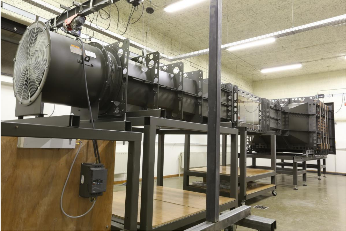
Standaert built a wind tunnel for testing Aeromodeller 2 shapes.
