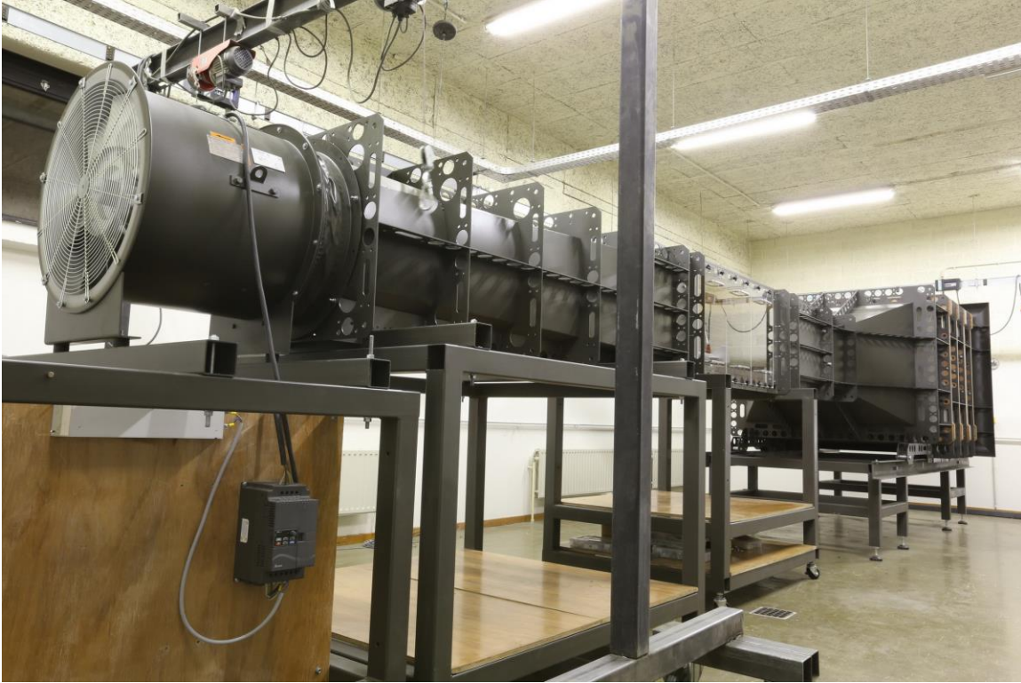
Standaert built a wind tunnel for testing Aeromodeller 2 shapes. Source: www.aeromodeller2.be
