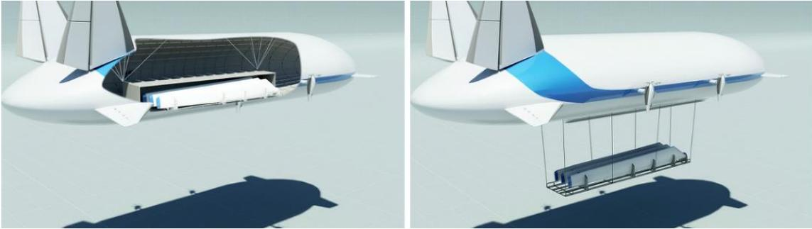
*Discharging cargo from a hovering Aeroscraft airship.
