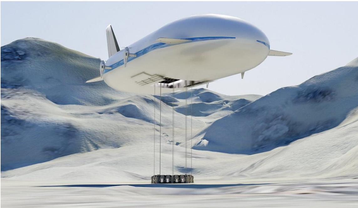
*Concept drawing, ML866 / Aeroscraft Gen 2 hovering and making an in-flight load exchange in the Arctic. Source: Aeros*
