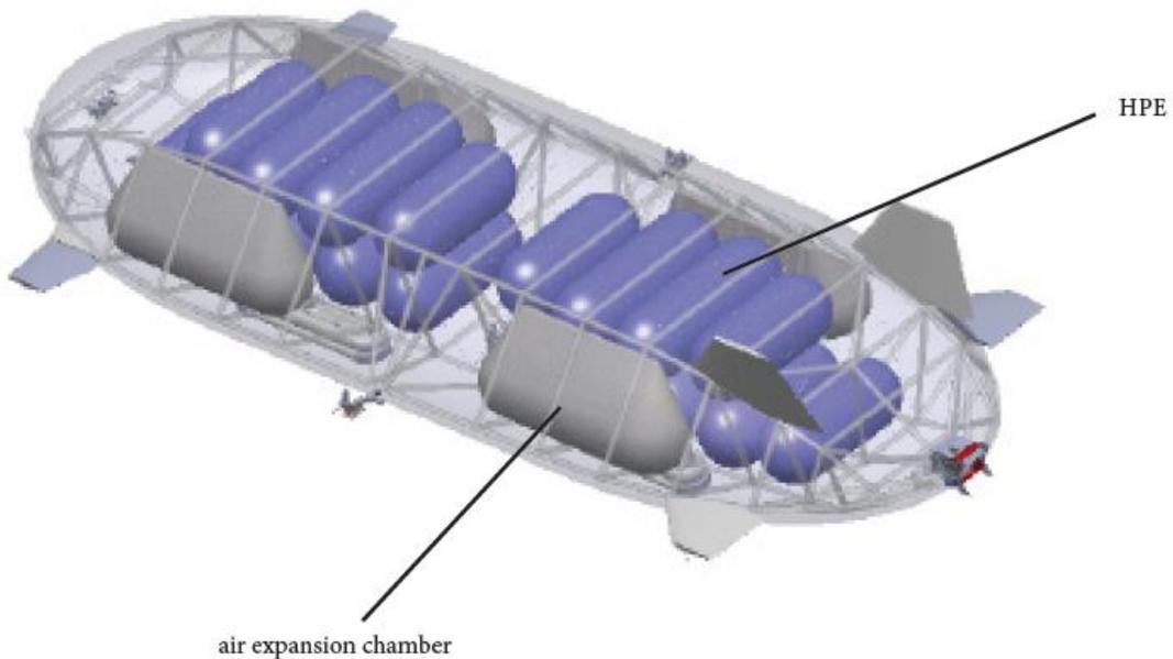
*Aeroscraft cutaway showing HPE and AEC. Source: Aeros*
