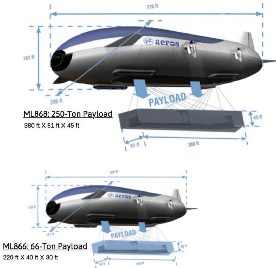
*Aeroscraft airship scaling to handle larger cargo loads.
