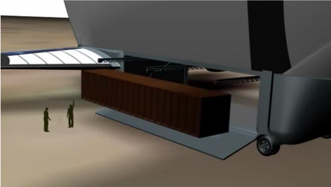
30 metric ton cargo capacity; cargo handling from side-mounted cargo bays. Source: Screenshot from video
