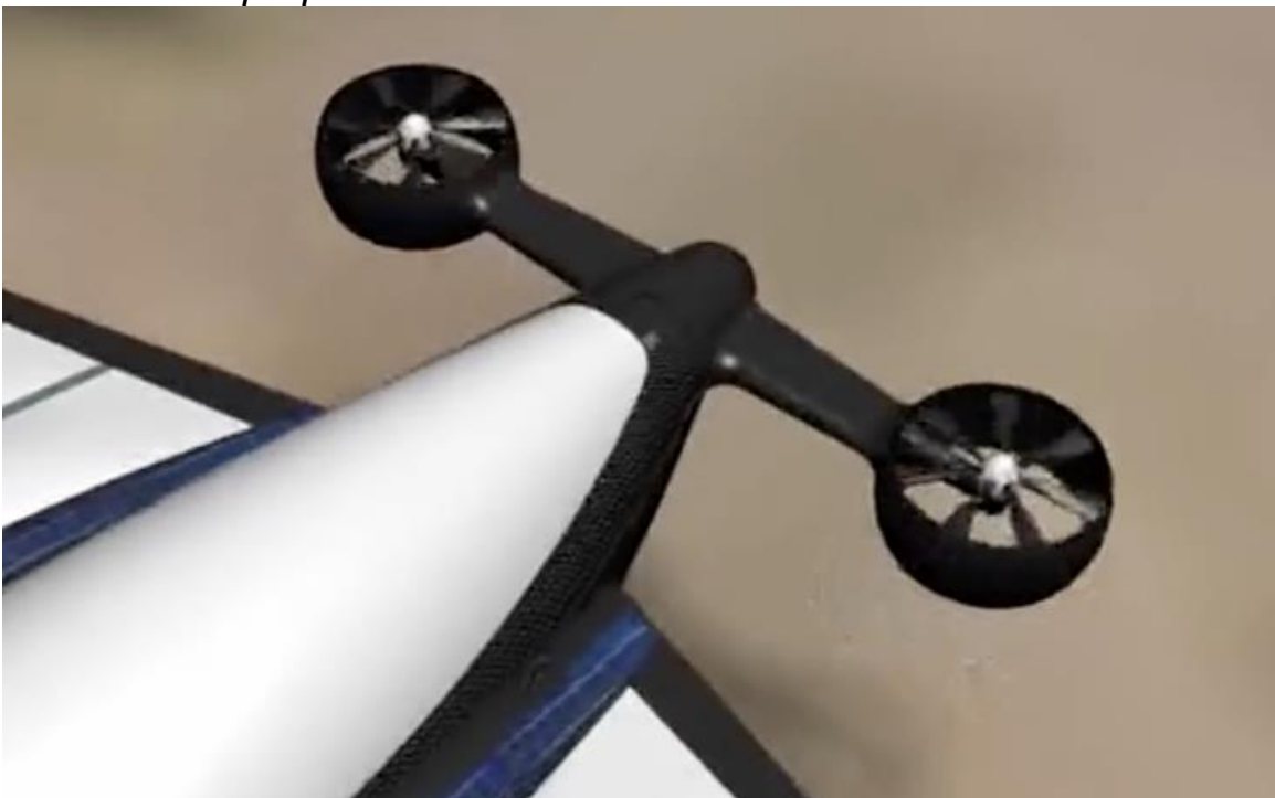
The stub wings supporting the rear thrust vectoring propulsors. Source: Screenshot from video
