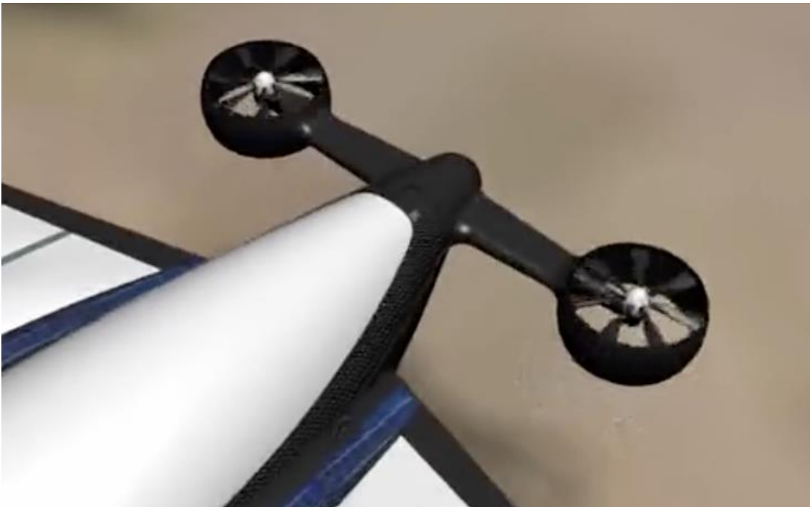
The stub wing supporting the rear thrust vectoring propulsors has limited rotation about the longitudinal axis of the airship. Source: Screenshot from video
