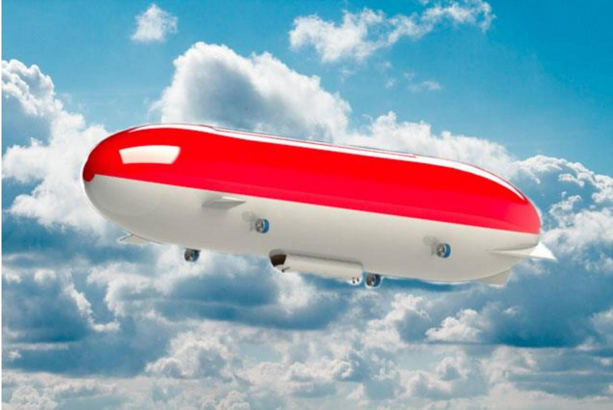
*Rendering of a BASI 30-ton MB 560 cargo airship in flight. The enclosed cargo bay is located under the center section of the gas envelope.*
