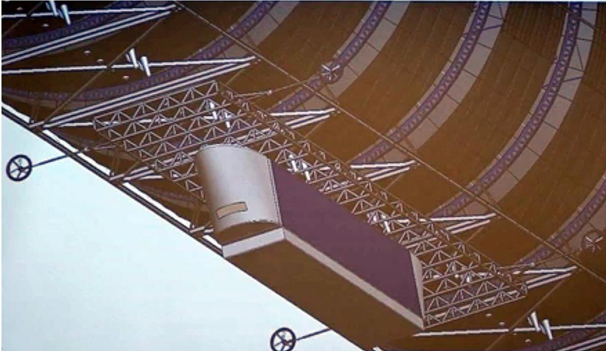
Arrangement of the gondola, including the cargo bay, and the load-bearing structure under the lifting gas cells. Source: BASI
