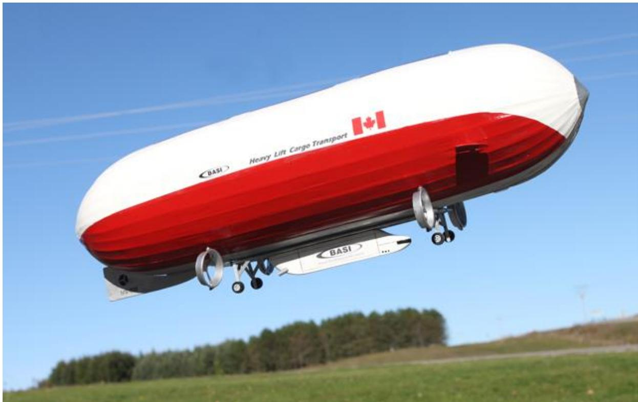
*1:100 scale model of the BASI airship. Source: BASI*
