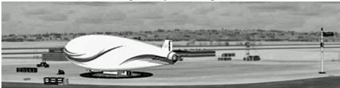
Rotating the turntable to point airship's nose in the direction of wind
