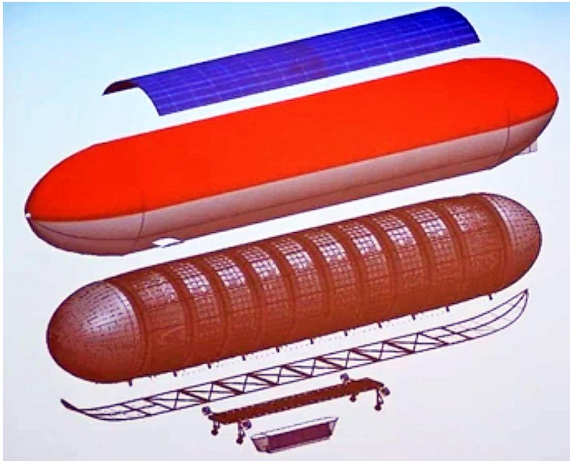
*Exploded view of the BASI 30-ton MB 560 cargo airship.
