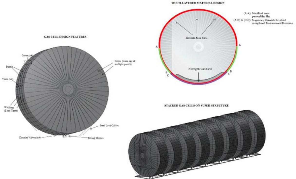
Low-permeability lifting gas cells, designed for helium or hydrogen. Source: BASI
