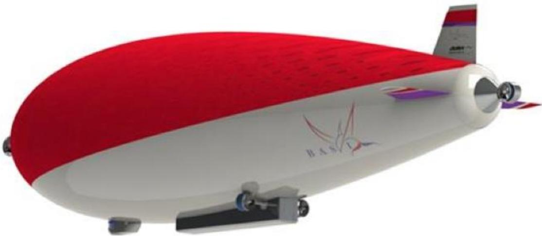
*Rear quarter view of an MB 310 airship showing the gondola and cargo bay along the bottom of the gas envelope. Source: BASI.*
