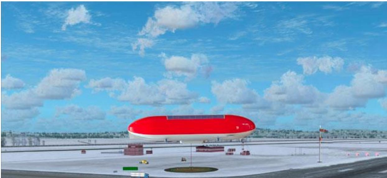
*Rendering of a BASI 30-ton MB 560 cargo airship being winched down to the landing pad on a Terminal Support System Buoyant Aircraft Rotating Terminal (BART). Source: BASI*
