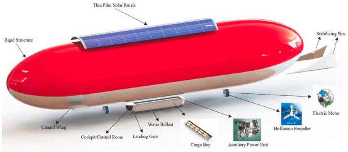
*Basic design features of the BASI 30-ton MB 560 cargo airship.
