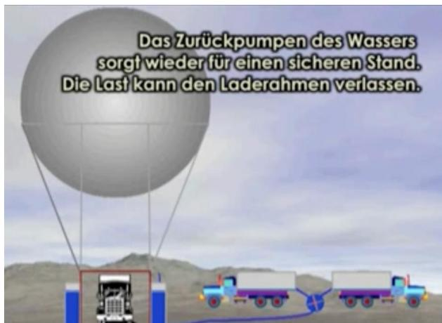
Pumping the ballast water back into the loading frame upon landing secures the balloon system safely on the ground. The cargo now can be removed from the loading frame. The balloon system remains held to the ground by the weight of the ballast water.
