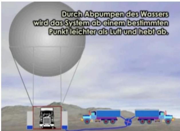
Pumping the ballast water from the loading frame to the tanker trucks makes the balloon system lighter-than-air and it lifts off at a certain point with the cargo.
