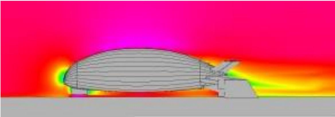
*Visualization of airflow around the hull of a DS 1500 on the ground. Source: Dirisolar.*
