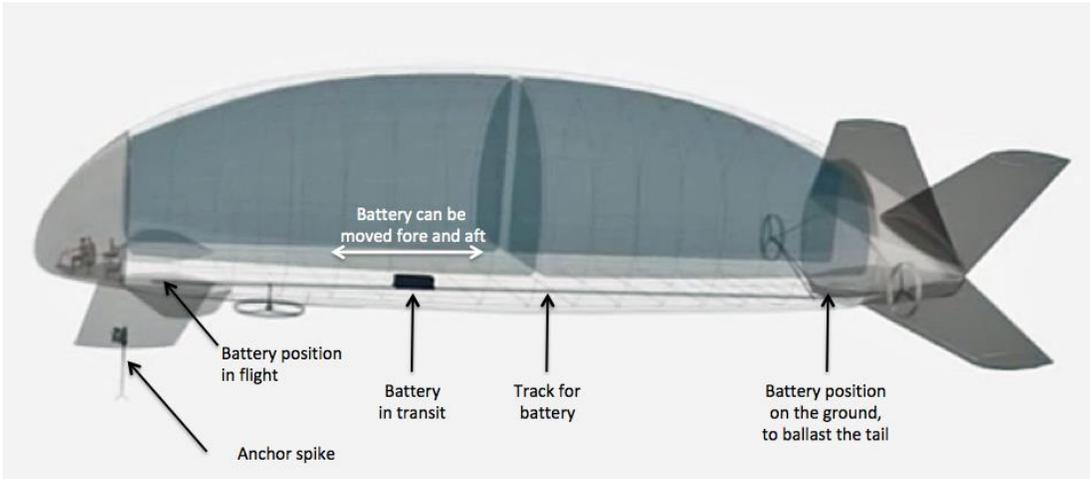
DS 900 airship internal arrangement shows the movable battery.
