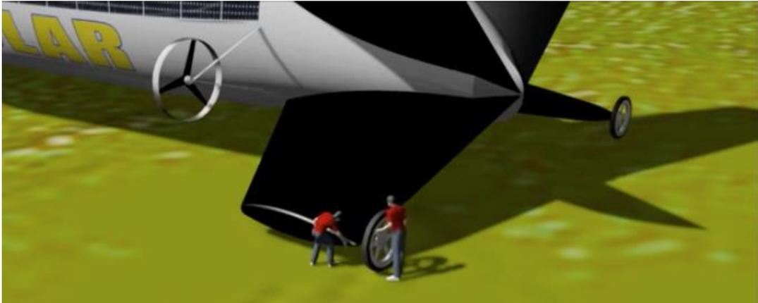
Wheels attached to the rear stabilizers after landing.
