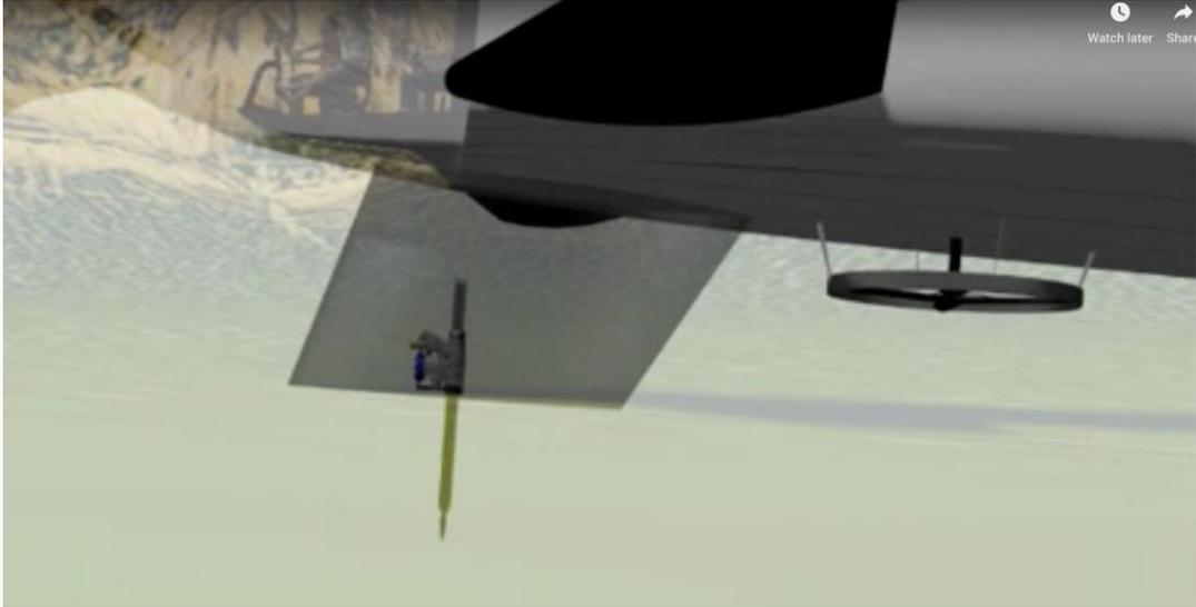
An anchor in the nose fin penetrates the ground after landing.
