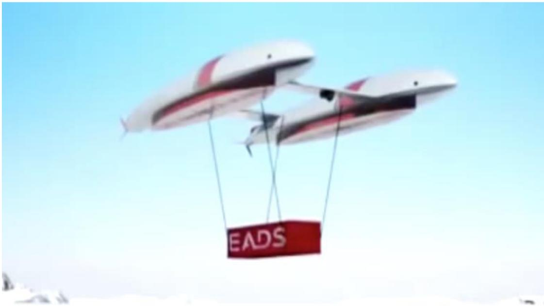
*Airship carrying an external load. Source: EADS*
