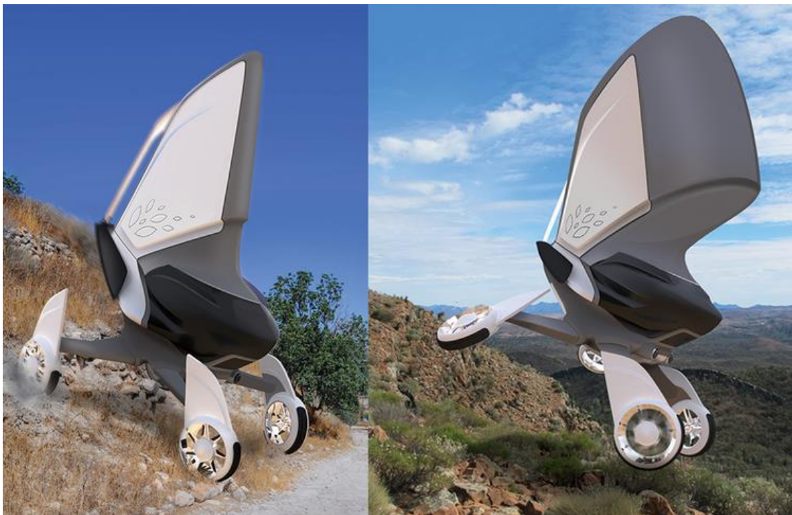
Escape traversing rough terrain (left) and in flight with the gas envelope expanded (right)
