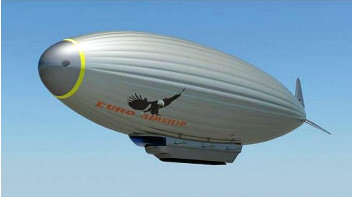
*Front quarter view of a DGPatt airship. Note the placement of the bow lateral thruster and the propulsion propellers along the side of the gondola.
