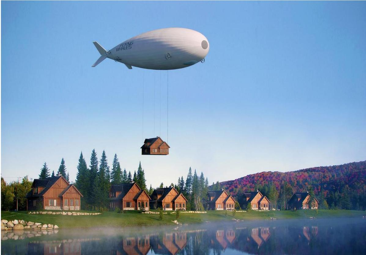
*LCA60T shown delivering a complete housing unit as an external sling load. Source: Flying Whales*
