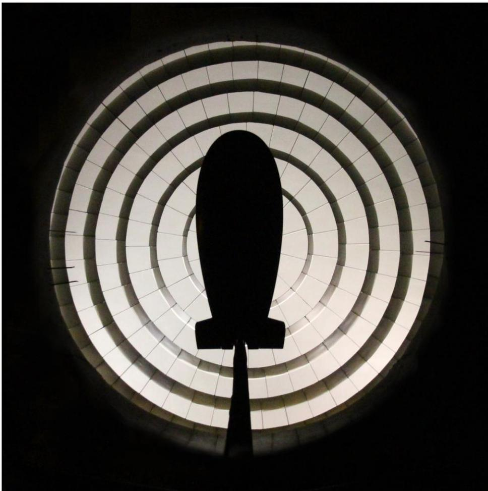
*LCA60T model in an ONERA wind tunnel.*
