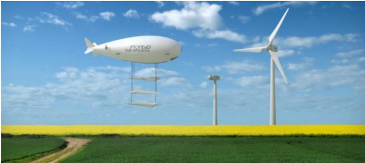
*LCA60T shown delivering a set of wind turbine blades as an external sling load. Source: Flying Whales*
