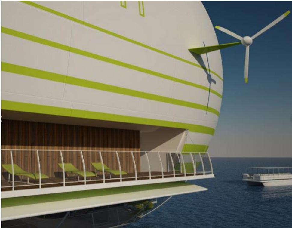
*The open-air balcony above the pressurized passenger deck is deployed when the Flying-Yacht is on the water. Note the electric motor-driven propulsor and the small stub wing. Source: octuri.com*
