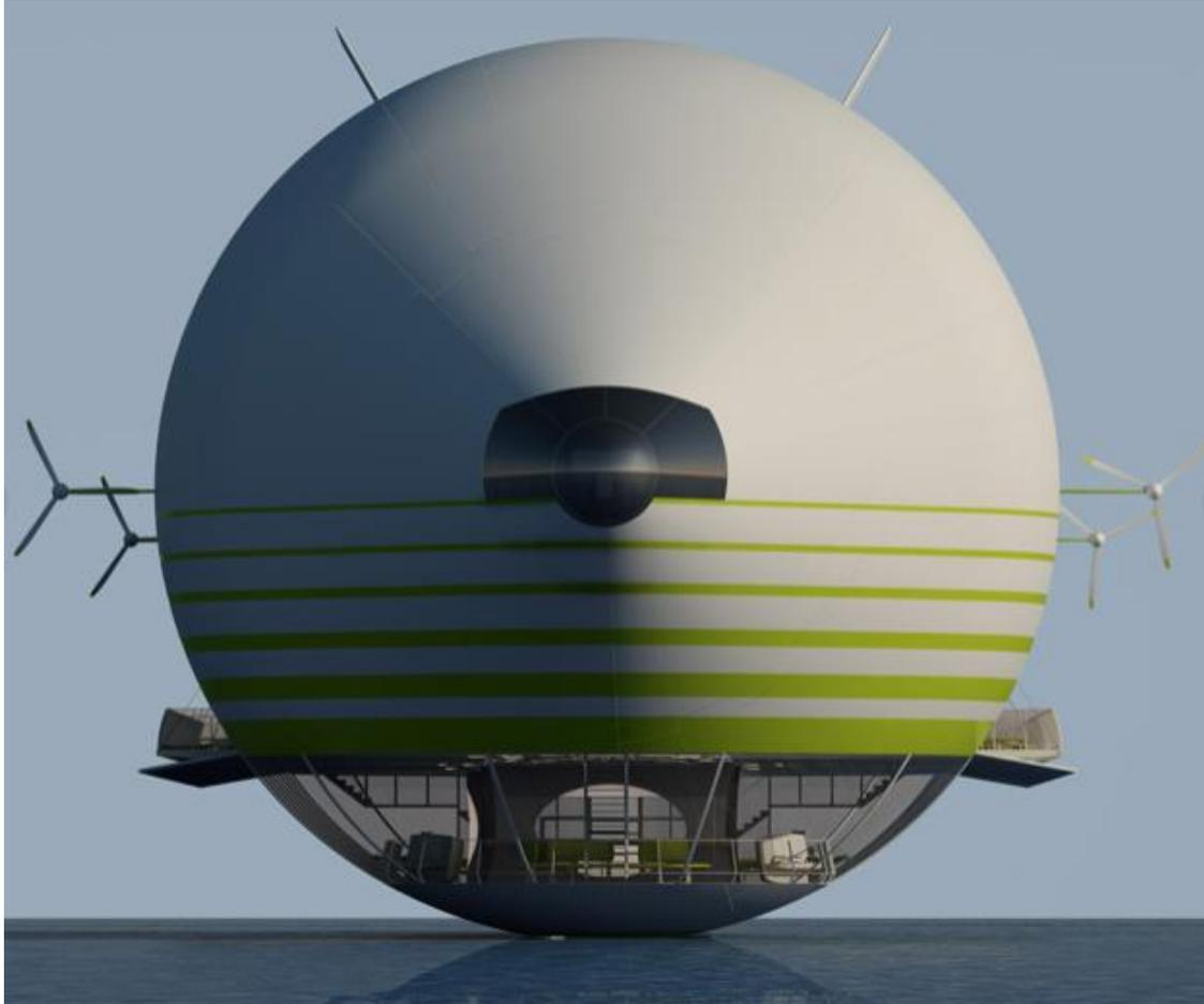
*The pilot station is in the nose of the craft. Note the four propulsors and the open-air balcony above the pressurized passenger deck.*
