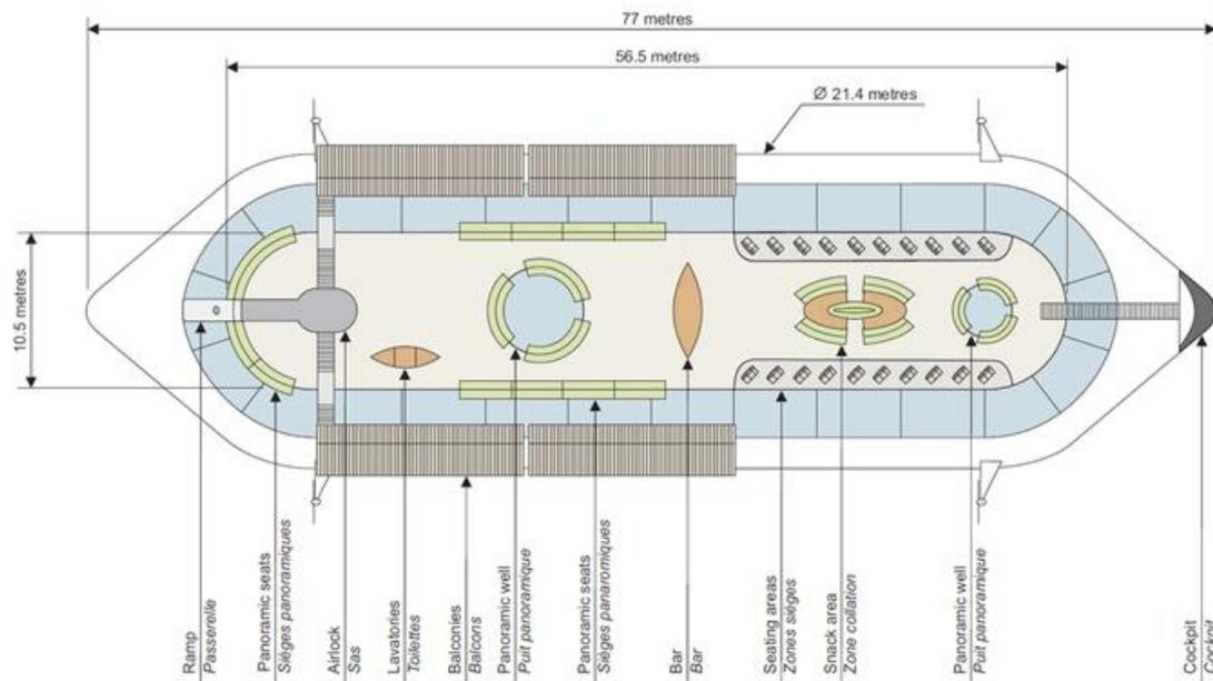
*Open floor plan of the passenger deck. Source: octuri.com*
