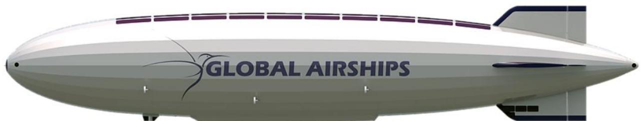
*Profile view of the Atlas airship. The ventral crew cabin located forward of the mid-ships cargo hold contains the forward-facing piloting station and the rear-facing crane operator station. Source: Global Airships*
