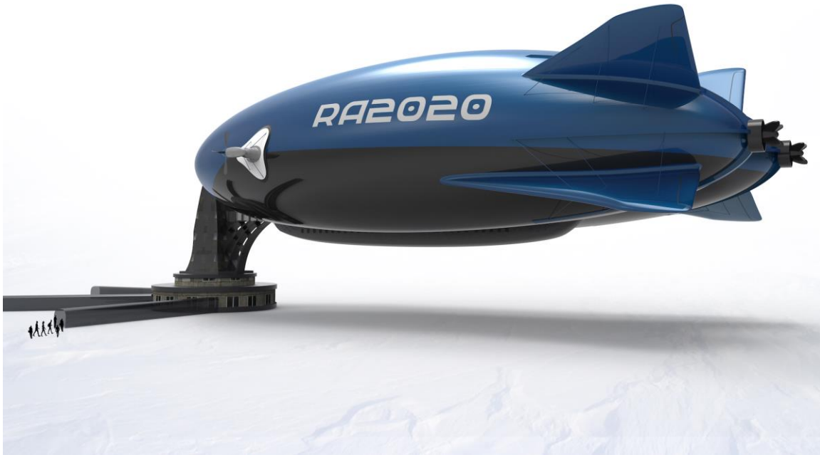
Aerostratos secured to a low mooring station. Source: Imaginative
