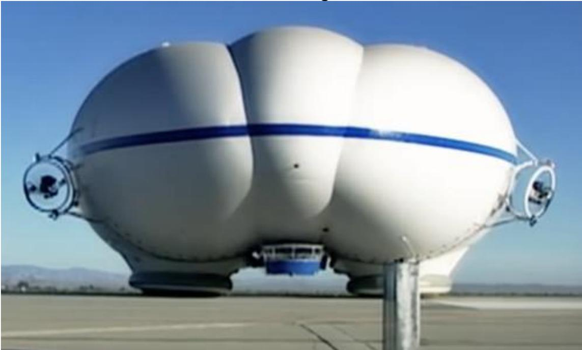
*Bow view of the P-791 showing the tri-lobe hull design and the two bow vector thrust units.*
