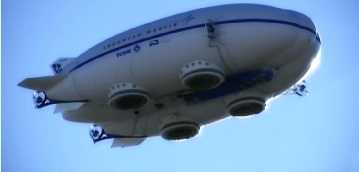
*P-791 showing the four ALCS units under the fuselage.
