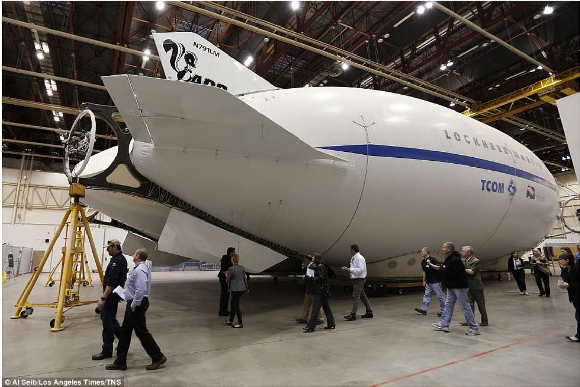
*Stern quarter view of the P-791 in its hanger showing the rear fins and one of two stern vector thrust units.*
