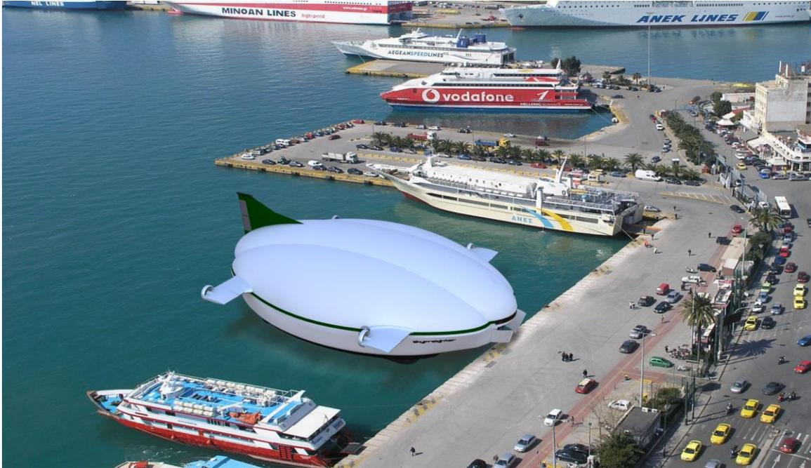
*SkyFreighter SF50T airship concept dockside, loading and unloading from a bow door. Source: Millennium Airship, Inc.*
