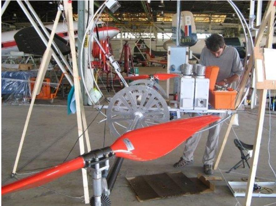
*One propeller and drive assembly. The battery is in the orange box. Source: Project Sol'R*
