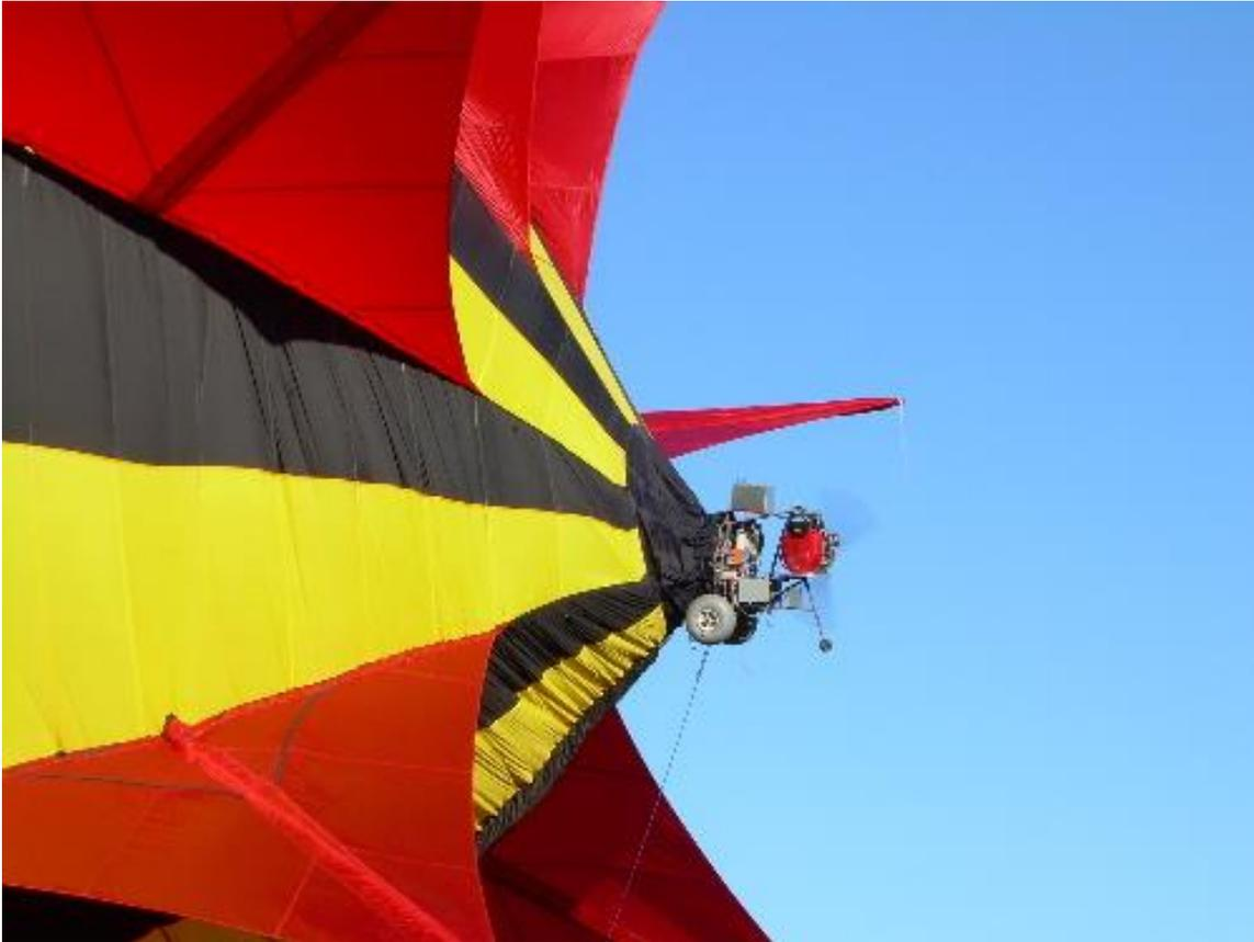
*A close-up look at the tail, showing that the engine has been rotated to the right (away from the camera), pushing the tail to the left and turns the nose of the aircraft to the right.*
