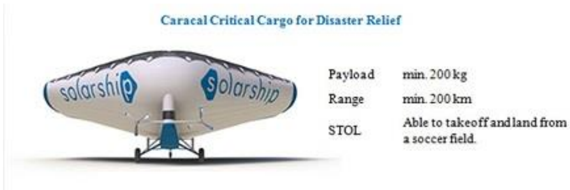
Original 20-meter Caracal prototype design, circa 2016. Source: Solar Ship
