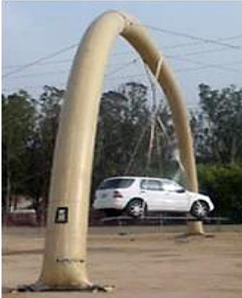
*TP Aerospace airbeam suspending a car.
