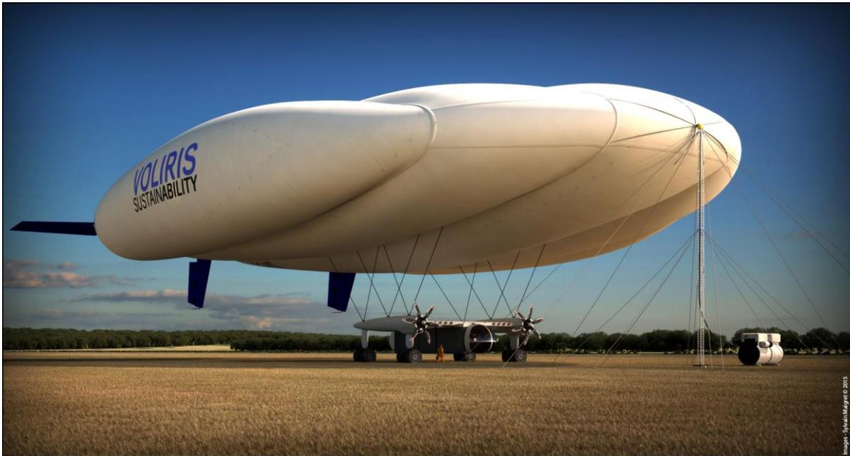
*Concept drawing of an NATAC V932 hybrid airship on the ground, connected to a mooring mast. Note the suspension lines connecting the engine and landing gear nacelles to the buoyant envelope.*
