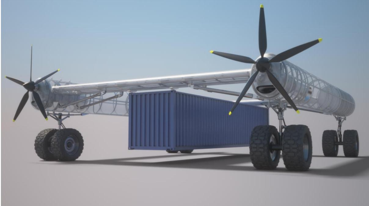
*Details of the NATAC engine and landing gear nacelles and a centerline mounted standard 32T shipping container engaged by a container gripping module (CGM).
