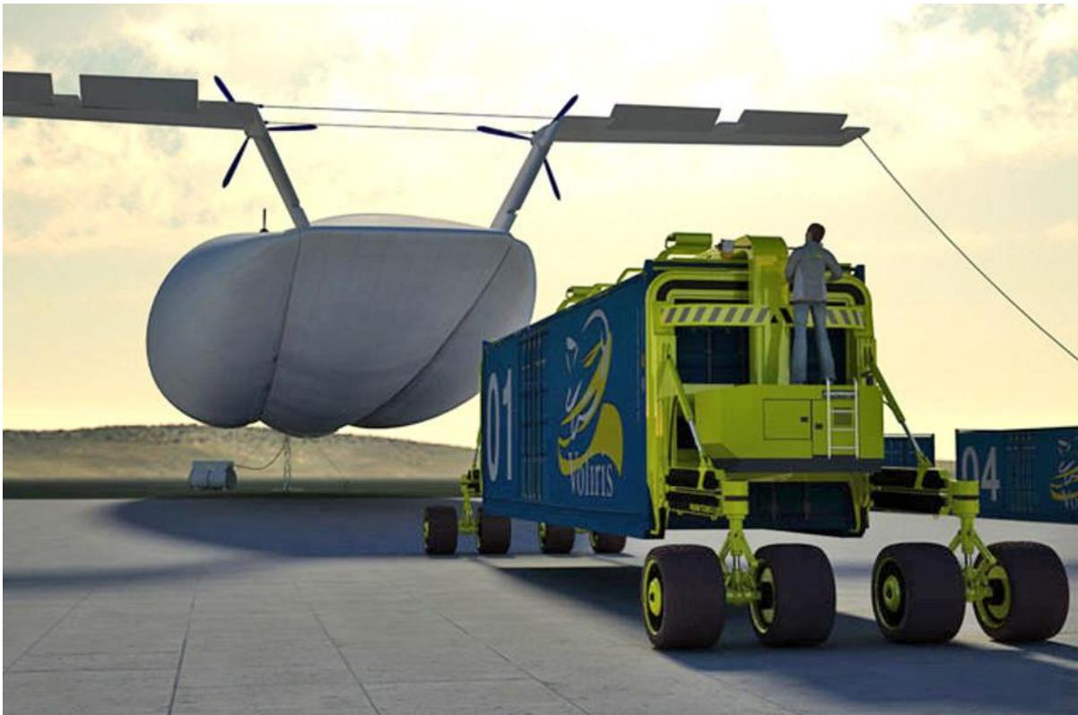
*Cargo container handling equipment for the V930. Source. Voliris*
