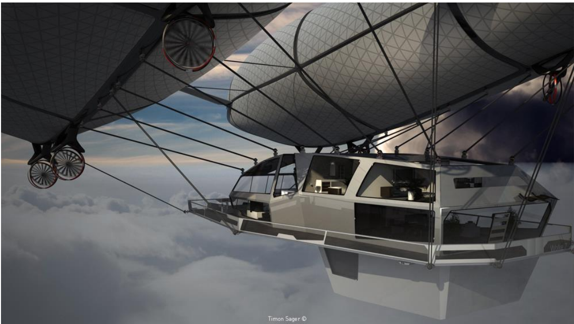
The passenger “gondola” (the house) is suspended between the two airship hulls.
