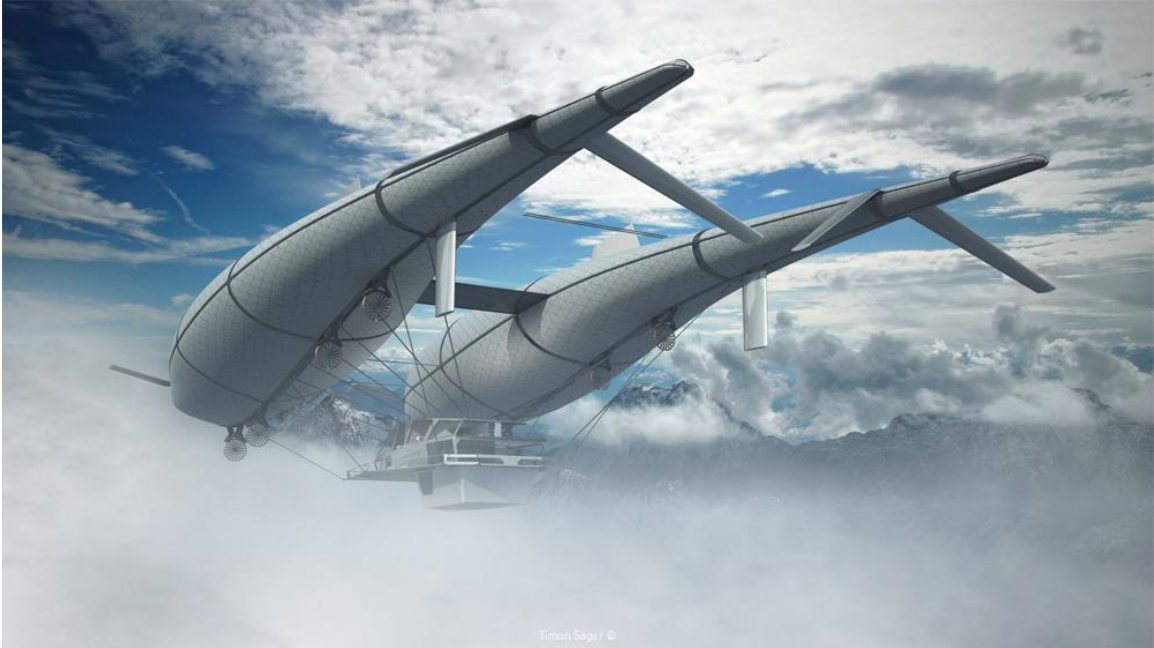
The passenger “gondola” (the house) is suspended between the two airship hulls.
