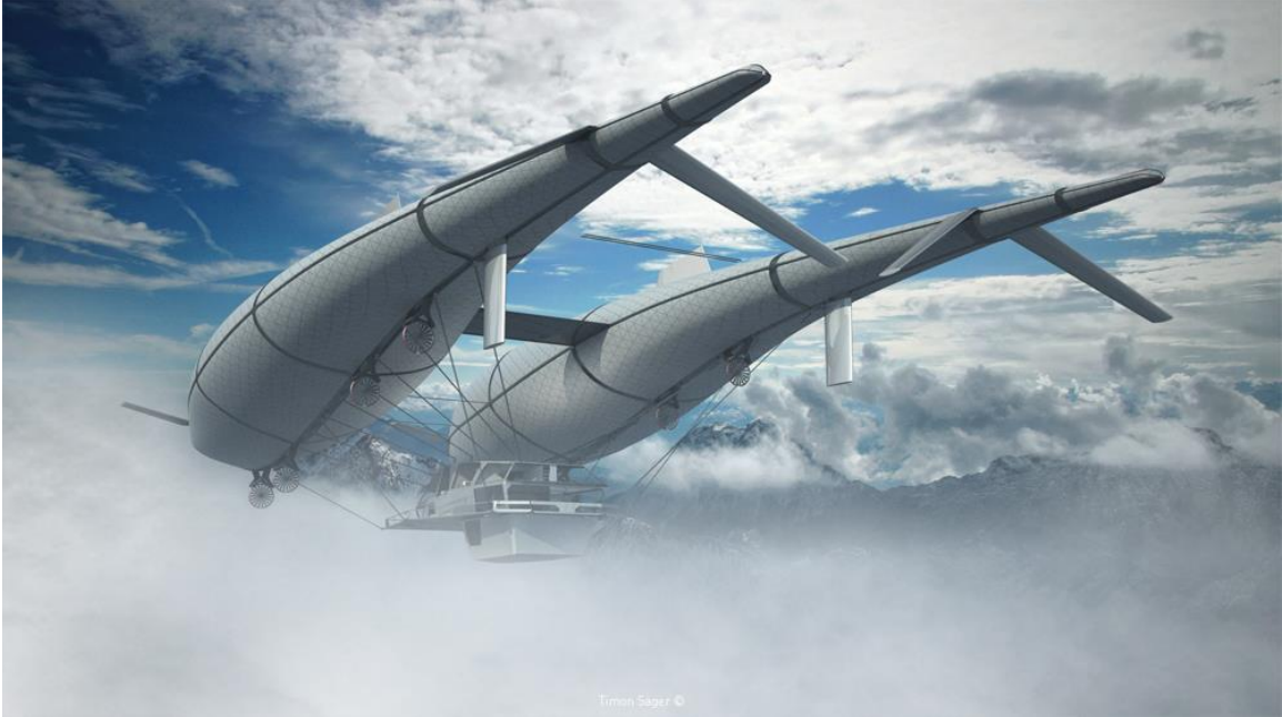
The passenger “gondola” (the house) is suspended between the two airship hulls.
