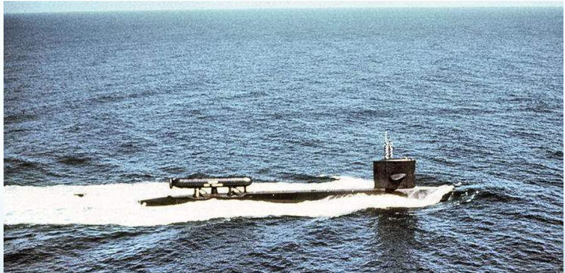
USS Parche circa 1983 (before hull extension). The “DSRV-look-alike” structure on the boat's aft section was a lock in-lockout chamber for saturation divers Source: www.navsource.org
