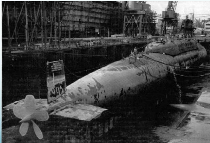
SSBN-598 in drydock. Note the 5-bladed propeller. Source: https://imgur.com/a/IQBOi
