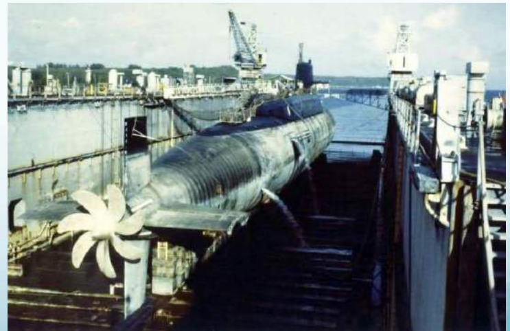
SSBN-599 in drydock. Note the 7-bladed "skewback" propeller. Source: http://www.shipmodels.info
