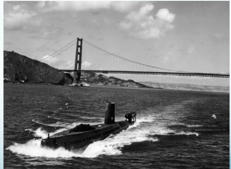
Halibut circa early 1970s with a DSRV-like saturation diving chamber on the aft deck and foredeck thruster removed.
