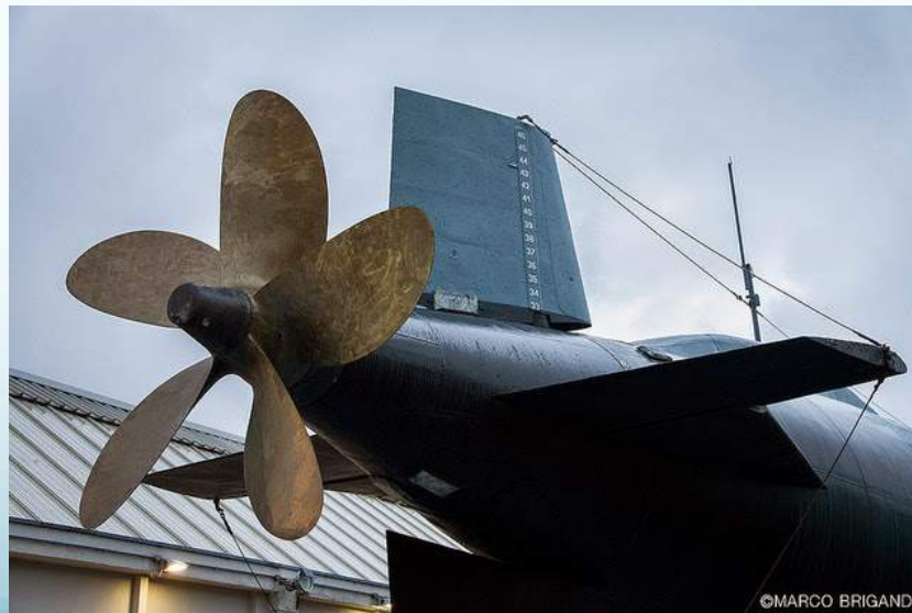
USS Tullibee 5-bladed prop
