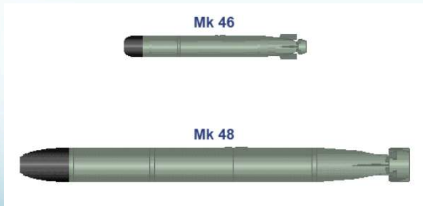
Relative size of the Mk-46 lightweight torpedo use in CAPTOR and the Mk-48 heavyweight torpedo.
