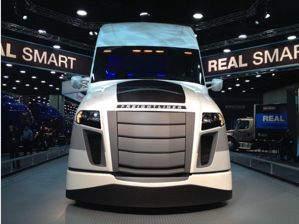
The Freightliner SuperTruck I with the active grill in the closed (high-speed, aerodynamic) position. Source: Daimler AG
