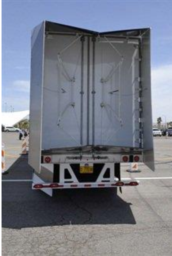
A commercially-available boat tail was installed on the trailer. Source: HDT Truckinginfo, 12 July 2015
