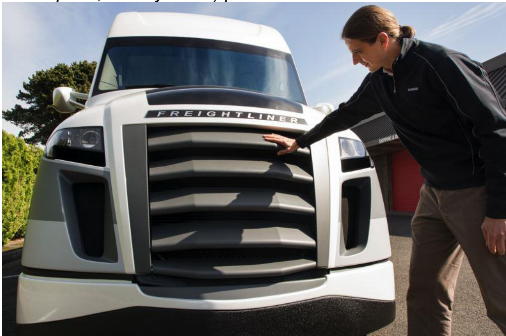
The Freightliner SuperTruck I with the active grill in the open (low-speed, high-torque) position. Source: Business Tribune, 28 April 2015
