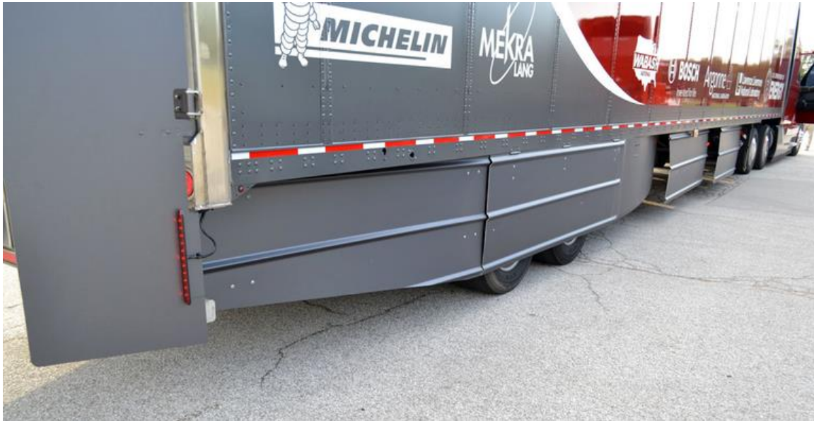
CataliST SuperTruck showing the slotted side skirts and the rear boat-tail (flow convergence device).
