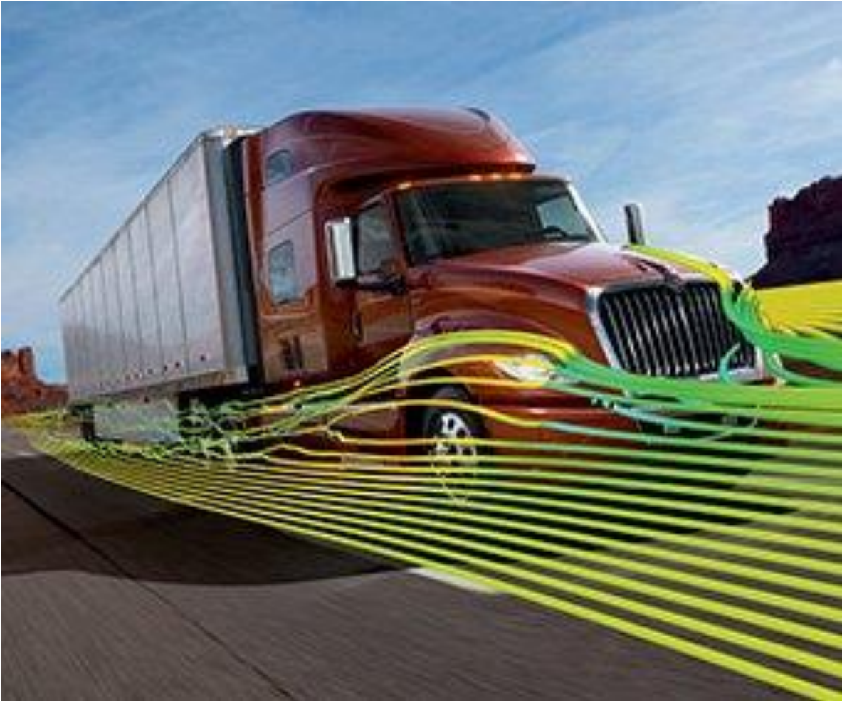
International LT-series tractor aerodynamics illustrated. Source: International / Navistar
