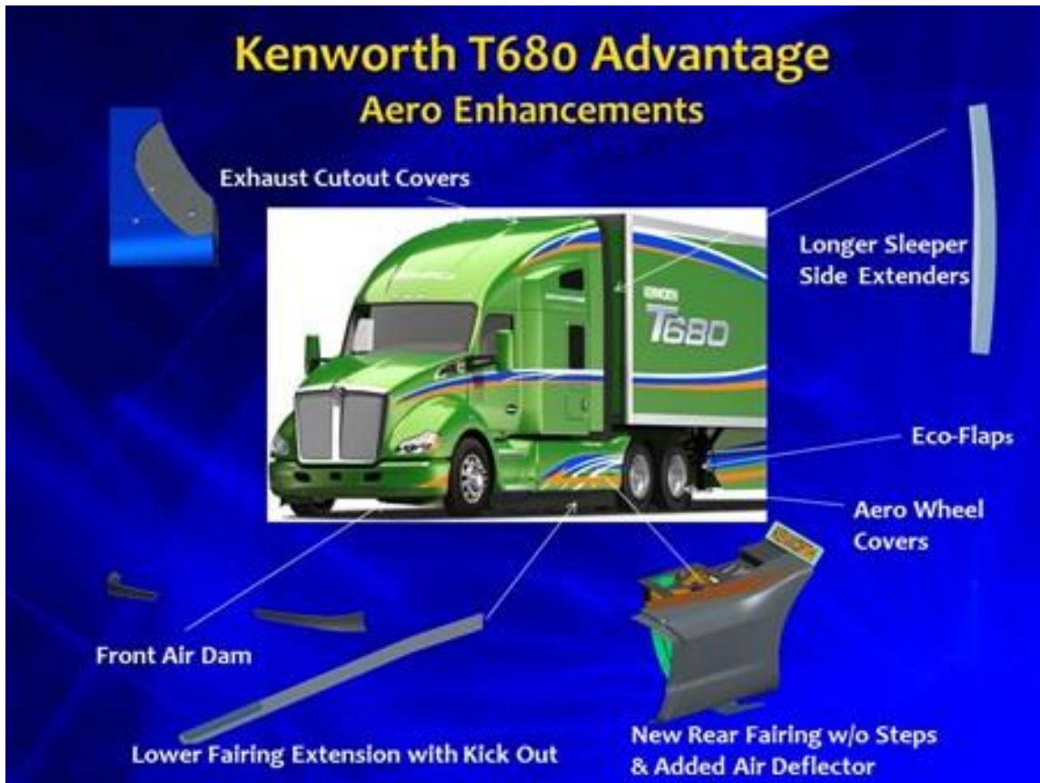
T680 Advantage aerodynamic improvements, circa 2014. Source: Kenworth
