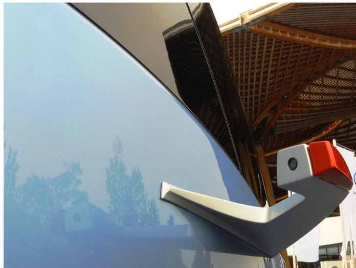
MAN Concept S tractor with Krone AeroLiner trailer at the IAA 2012 exhibition. Note the rear-facing video cameras replacing the side-view mirrors. Source, both photos: Spielvogel via Wikipedia
