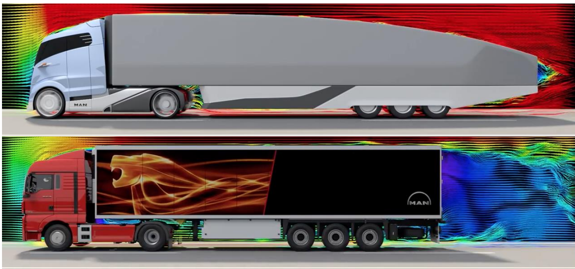
MAN aerodynamic comparison of the Concept S and a conventional European tractor-trailer, which has a large, low-pressure area (blue area) behind the rectangular trailer. Source: Screenshot from MAN video
