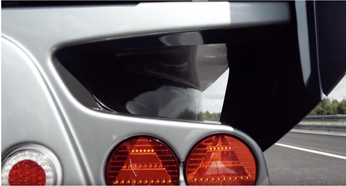
Details of the trailer rear diffuser.
