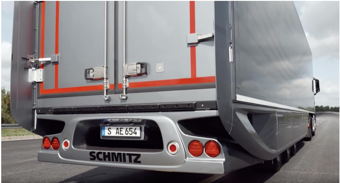
Details of the trailer side panels, rear diffuser and tapered, hinged fairing that extended the total vehicle length beyond the EU limit. Source: Screenshot from Daimler AG video, 2013
