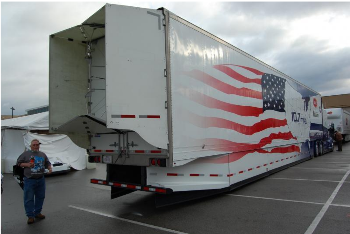
Aerodynamic boat-tail on the Cummins-Peterbilt SuperTruck I. Source: FleetOwner.com, 12 March 2015
