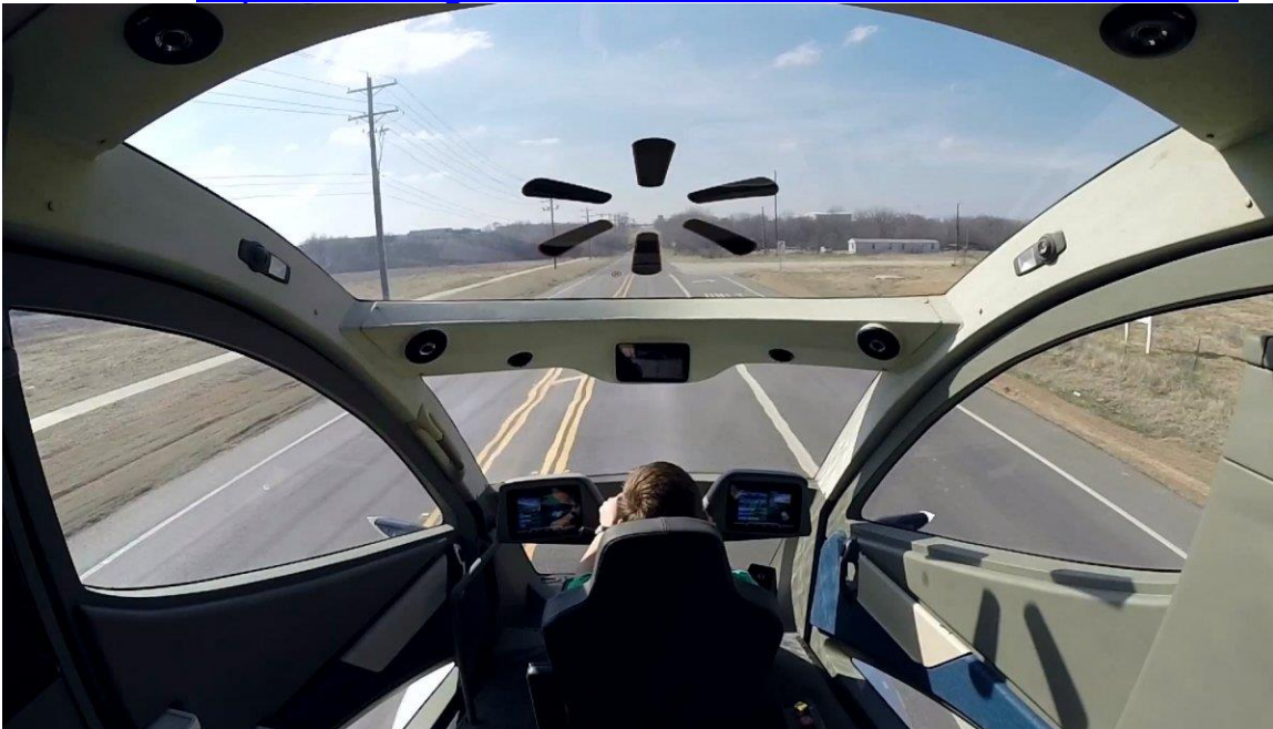
View from the cab. Note the center-mounted driver's seat flanked by digital displays. Source: Walmart
