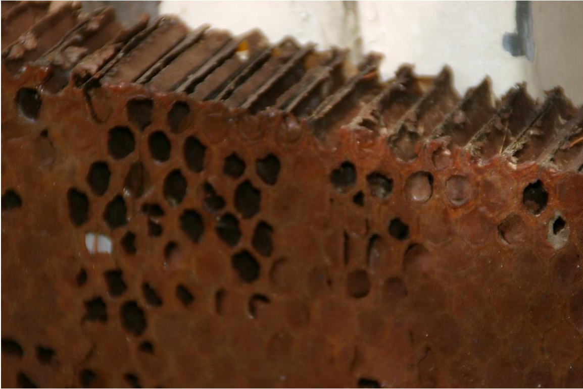
Original lumicomb honeycomb core section with the aluminum skin removed. Source, both photos: http://www.thefleethouse.com .
