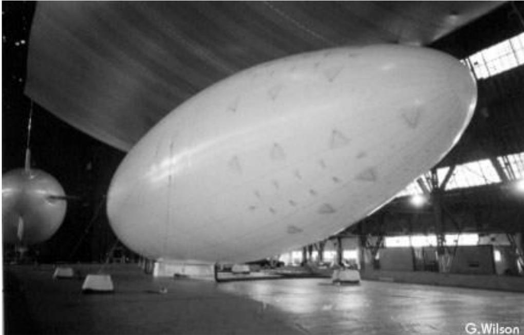
*StratSat's bare helium filled envelope was held down by heavy concrete blocks in a hanger at Cardington. The many triangular anchor points on the envelope mark locations that may carry a load.*
