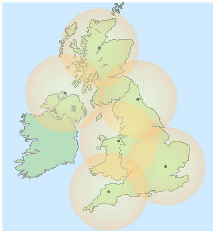
*Example of regional coverage for the UK with 6 HAP airships stationed at 20 km altitude with line-of-sight propagation between HAPs. Source: T. Tozer & D. Grace (2001)*
