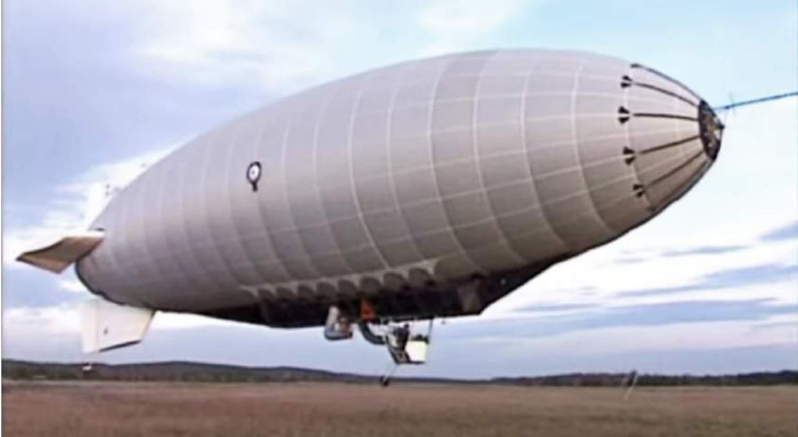
Joey on approach to landing. The black circle visible on the side of the envelope is one of two helium valves. Source: Screenshot, Joey-Testflug video (2008)
