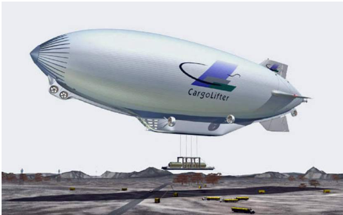
Load exchange in progress from a CL160 hovering at about 100m (328 ft). Source, both graphics: CargoLifter AG
