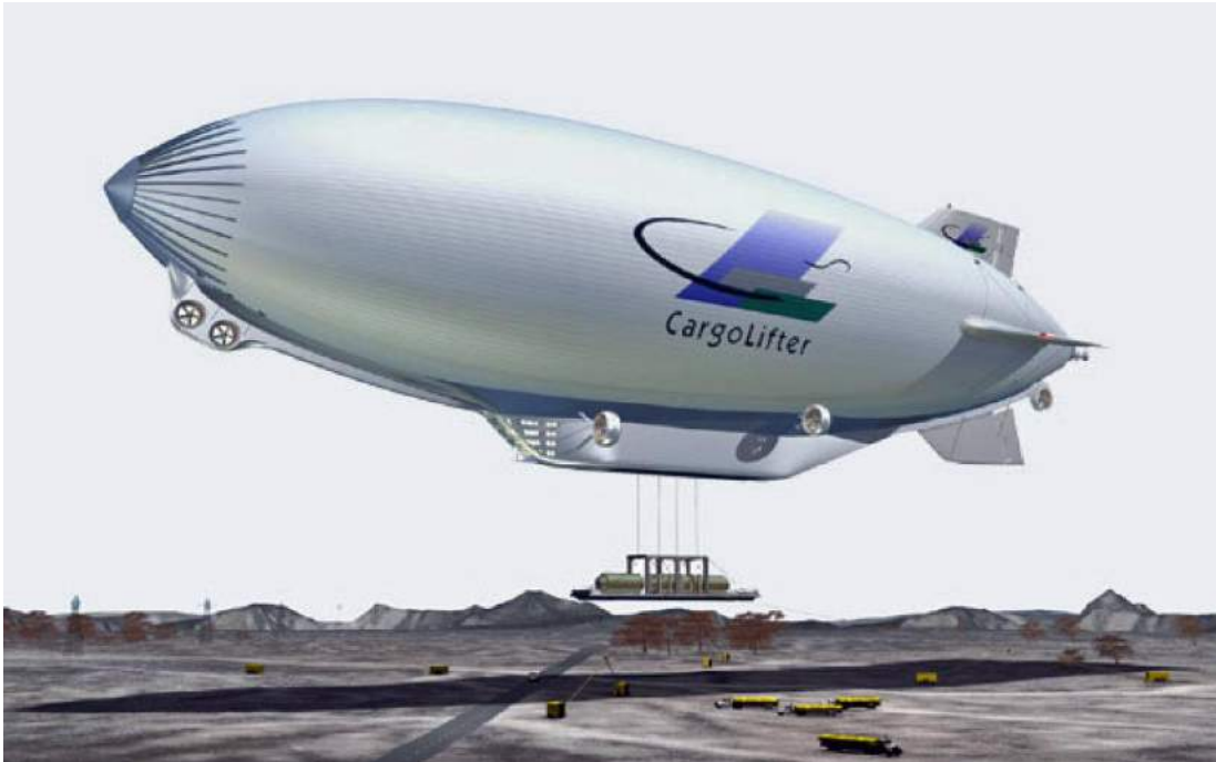
Load exchange in progress from a CL160 hovering at about 100m (328 ft). Source, both graphics: CargoLifter AG
