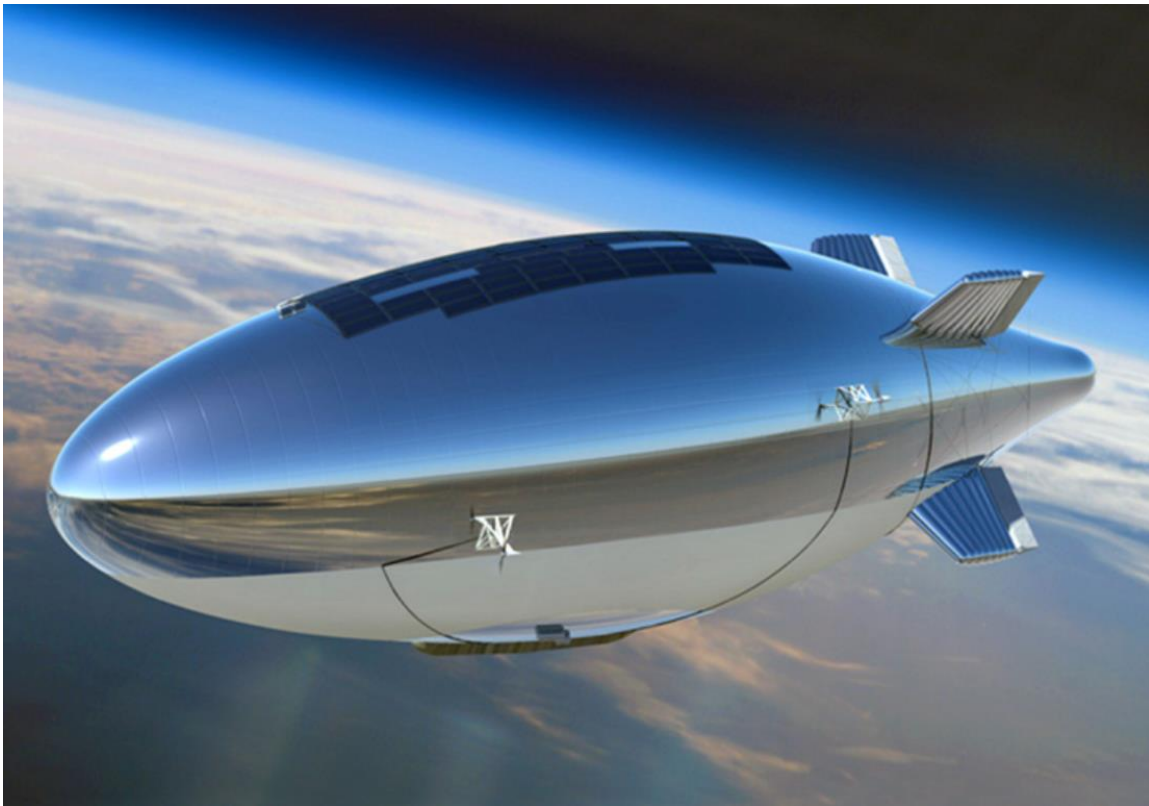
ISIS concept drawing showing solar panels and hull-mounted propulsors. Source: Lockheed Martin
