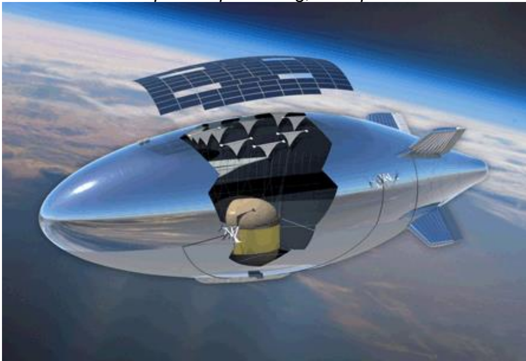
ISIS airship exploded view showing the location of the ASEA radar within the hull and the solar photovoltaic array on the top of the hull.
