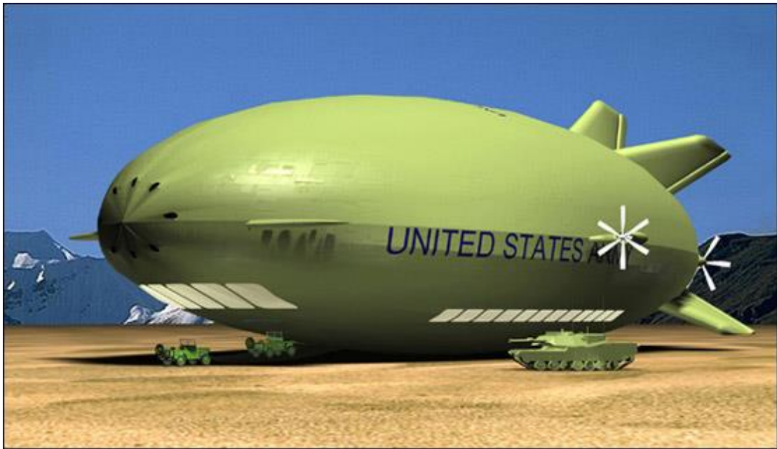
Aeros WALRUS variable buoyancy heavy lift airship concept. Source: Aeros via DARPA
