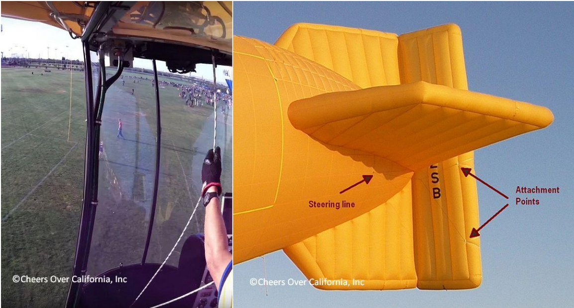
AS-105GD/4 controls for rudder & horizontal stabilizer. Source: http://www.cheersaerialmedia.com
