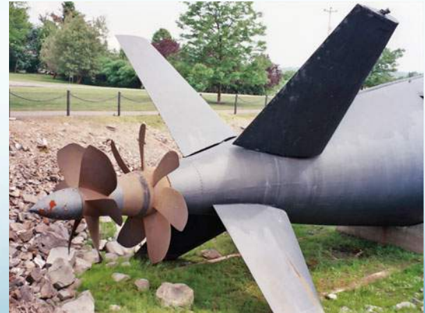
Below: Final X-tail & contra-rotating prop configuration
