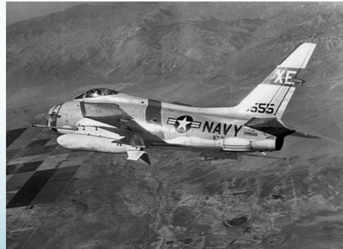
Mk-12 shape carried under the wing of a Navy FJ-4B Fury Source: US Navy photo / Wikipedia
