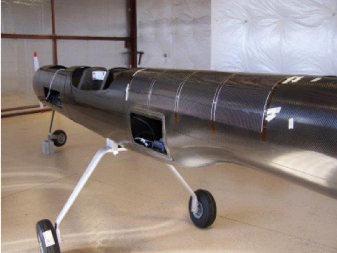
*Partially complete fuselage for the 40%-scale SRV demonstrator.
