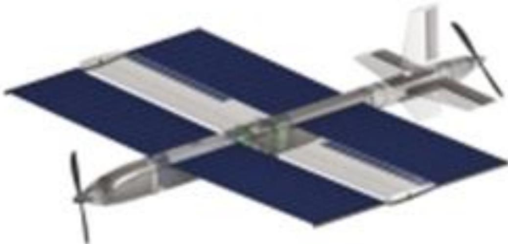
*General arrangement of the StarLight solar-powered SRV
