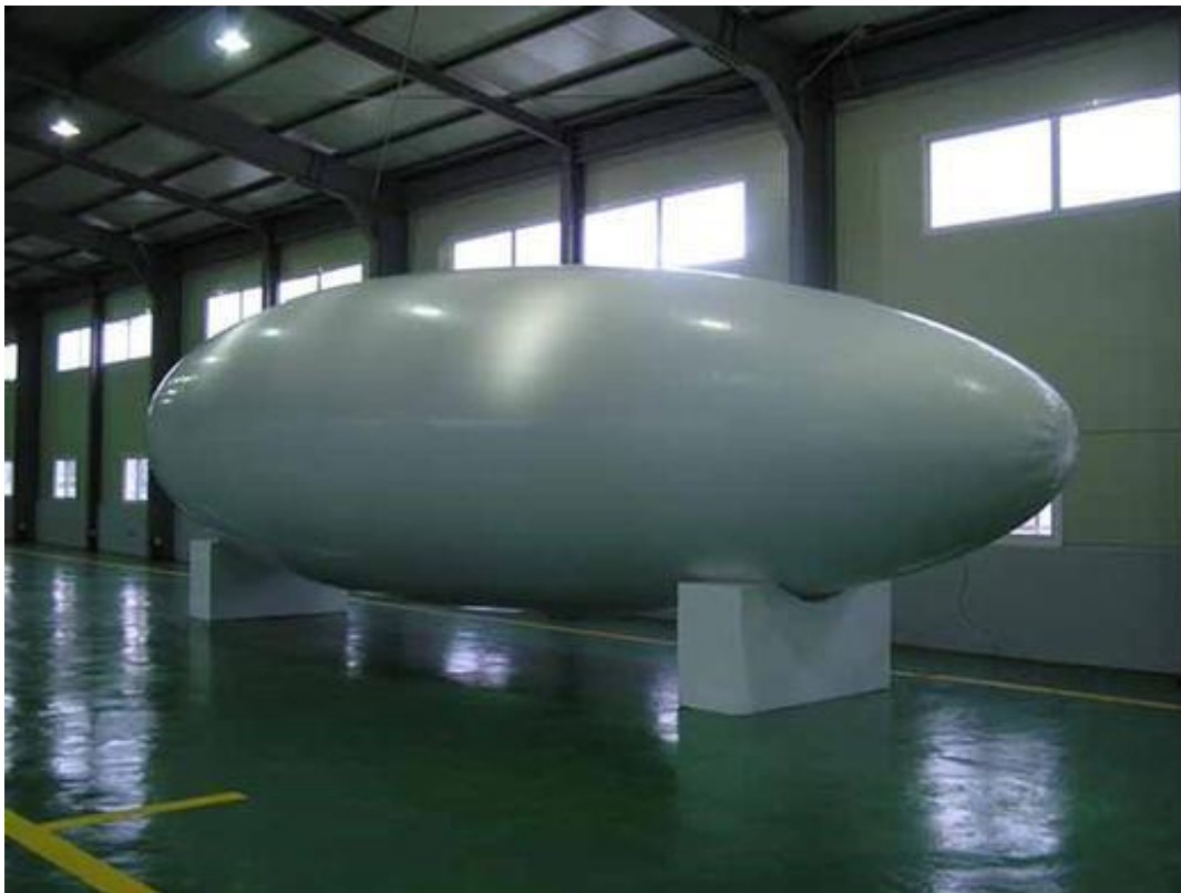
VIA-50 inflated hull before installing gondola, propulsors & tail fins. Source: Yung-Gyo Lee, et al., 2006
