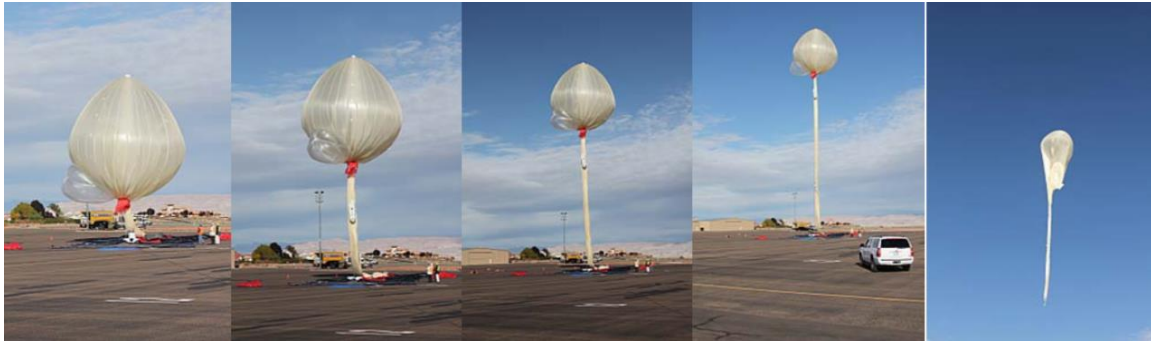
Partially-inflated HiSentinel 80 launch sequence.
