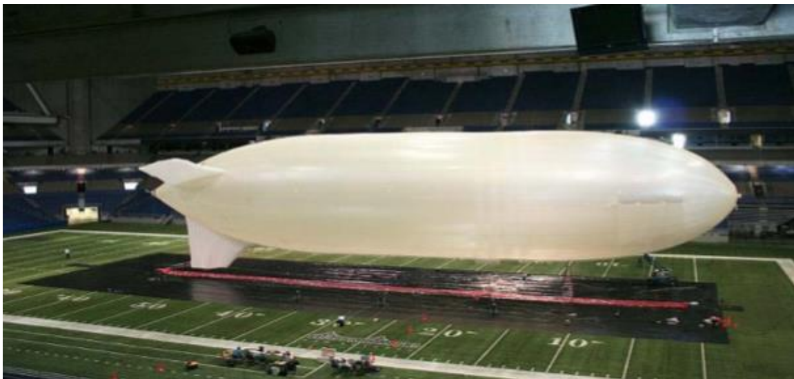
HiSentinel 80 inflation test in the Alamodome in San Antonio, TX. Source: Steve Smith Conference paper: DOI: 10.2514/6.2007-7748
